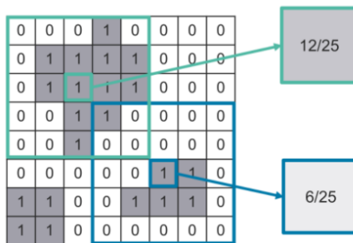
Figure 11. Illustration of the use of a neighbourhood of grid cells, in this case, a neighbourhood of 5 x 5 cells, to estimate the probability of an event occurring in the central cell when there is spatial uncertainty in the prediction
