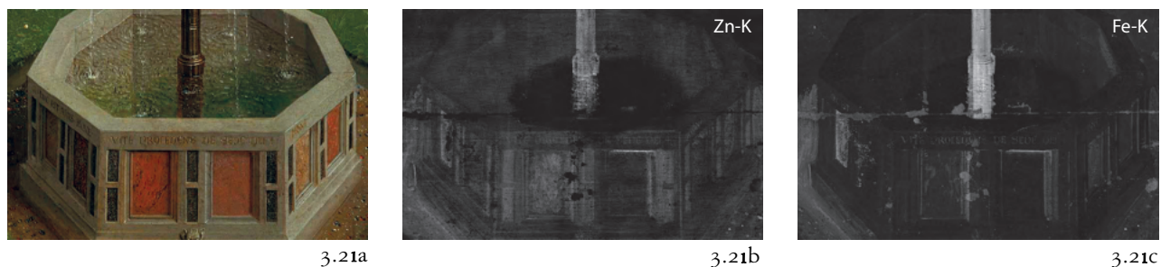
Fig. 3.21a–c. Adoration : detail of the lower part of the fountain with sampling location (a). MA-XRF distribution elemental maps for zinc (Zn-K) (b) and iron (Fe-K) (c) showing that the central brownish column is painted with a mixture containing an iron-based pigment(s) with quite high amounts of zinc additive.
