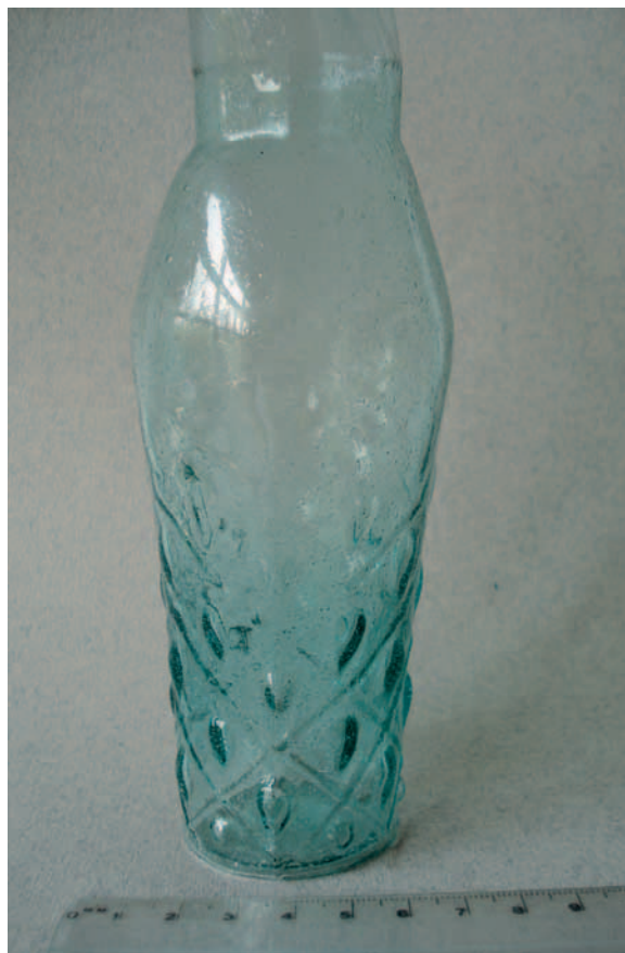
Fig. 14. An example of a beaker that is mis- shapen due to lack of air pressure during blowing. The upper bosses are faint and the moile is too narrow. © F. van den Dries.
