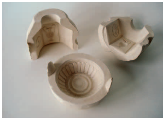
Fig. 2. Multi-part mould for a Syrian bottle, 'direct system'. © F. van den Dries.
