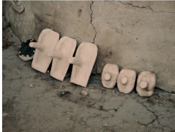
Fig. 17. Pre-heating of mould parts before use, placed against the hot wall of the furnace. To the left are mould parts for a Hercules' club beaker; to the right are parts for a Syrian bottle. © F. van den Dries.
