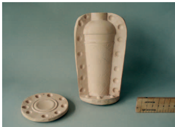
Fig. 3. Base and one wall section (of three), 'patrix-matrix system'. © F. van den Dries.
