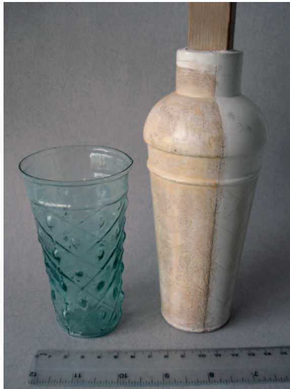
Fig. 1. The finished Hercules' club beaker, with slightly ground rim, next to the plaster master mould. Notice the difference in height and width. © F. van den Dries.
