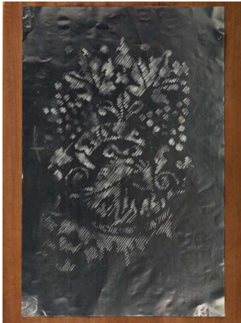
40b. The tin foil is beaten into the mould
