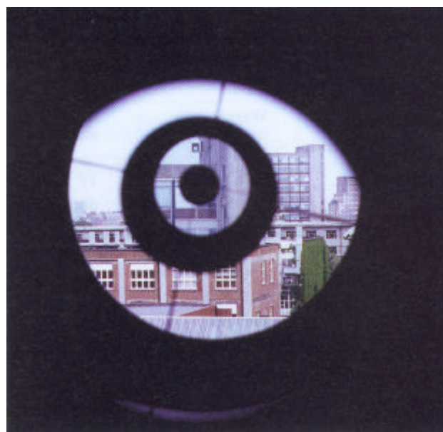
Fig. 2.1 - View through the emitting telescope of an 800 m atmospheric absorption set-up installed on the campus of the University of Brussels. The reflecting mirror can be seen on the opposite building (Photo P. Hannaert, Journal "Le Soir")
