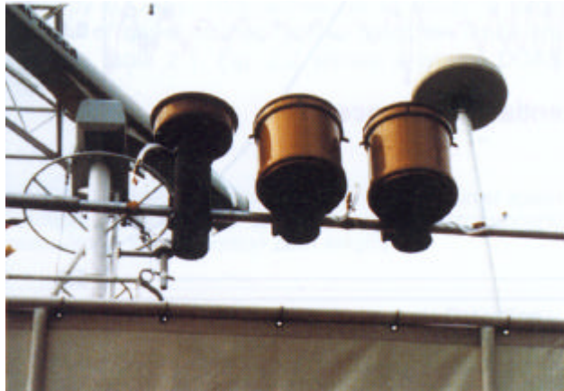
Fig. 2.3 - Two stacked filter unit (SFU) aerosol sampling heads (under orange rain covers), installed by the University of Gent group on the German research vessel Alkor during the Lagrangian North Sea Experiment (NOSE) in September 1991
