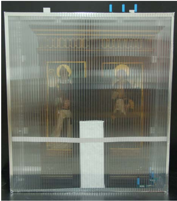
III. 2. Experimental setup to test the extent of pollution buildup in an airtight box ( \pm 100 \times 115 \times 40 cm) with EG3 ( \pm 90 \times 109 \times 30 cm) ©W.Anaf
