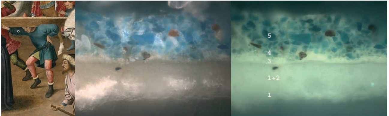
23 Cross-section from the blue drapery of the carrier of the Cross. Note the isolating layer, impregnating the upper part of the ground (1 and 2), followed by the imprimatura (3), and two blue layers, the first (4) containing finely ground azurite (10-20 \mu\text{m} ) and the second (5) coarsely ground azurite (20-50 \mu\text{m} ). Photographed at a magnification of 1000 \times .
