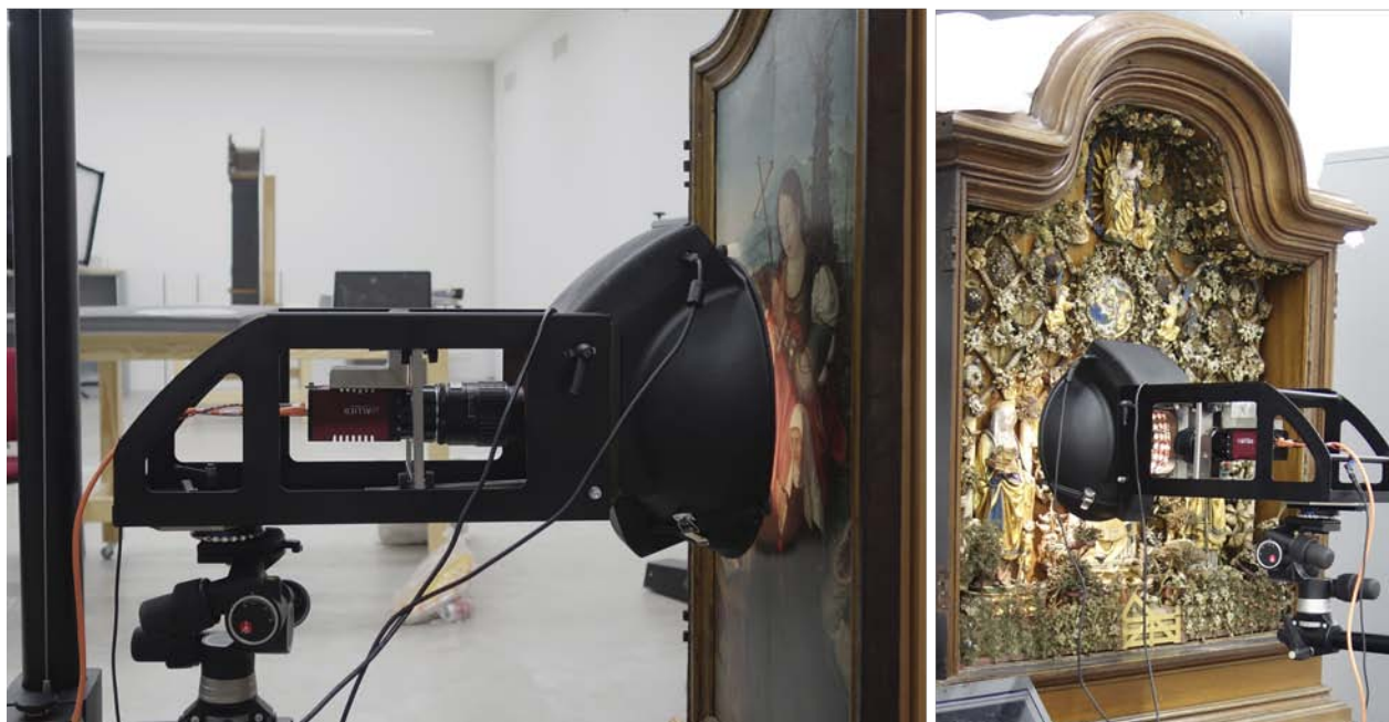
III. 2. Imaging of the Enclosed Garden of St. Ursula with the WL minidome (left) and the panel with St. Margaret with the MS microdome (right), mounted on a large horizontal copy stand © KU Leuven
