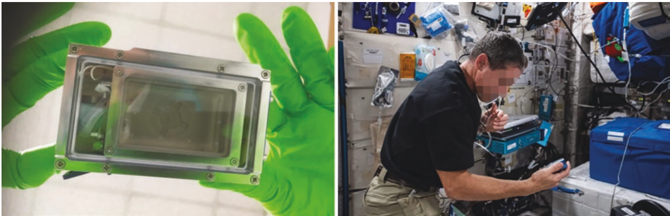
Fig. 10.21 View of one Rob2 hardware used onboard of the ISS (left) and Astronauts checking the correct rehydration of A. vaga individuals. Sixteen pieces of hardware were sent to ISS, each containing 40,000
