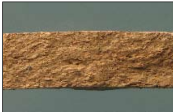
Figure 55: fresh break of a Maasland jar from the kiln at Heerlen
