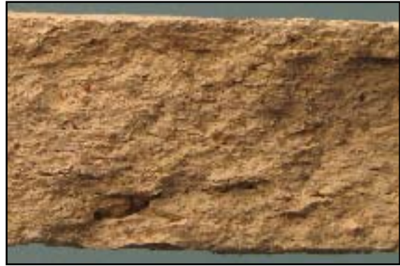
Figure 17: fresh break of a MAAS2 mortarium
