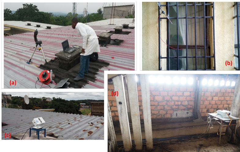
Figure 3.7: Installation of the instrument in Kinshasa. (panel a, b: MAX-DOAS measurement with version 1) (panel a, b: scanner on the roof of UniKin’s Faculty of Science and the control and command unit : version 2)
