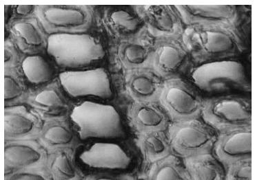
Figure 5: Micrograph cross section of the decayed zone of a beam extracted from the Zonnebeke Church Dugout showing features related to decay types.
