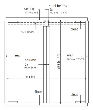
Figure 6: Structure of the central tunnel of the Zonnebeke Dugout (Ingenieursbureau Norbert Provoost byba)
