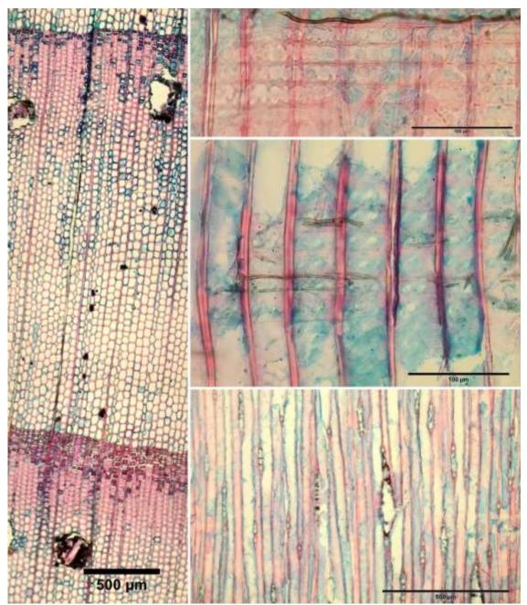
Figure 2: Thin sections of *Pinus banksiana* timbers from the Zonnebeke Church dugout. Transverse section with resin canals (left). Dentate inner cell walls of the ray tracheids (upper right). Pinoid pits in the cross fields (central), and ray of 3-1à cells high (lower right).
