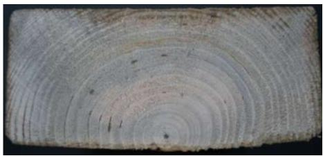
Figure 4: Cross section of a beam extracted from the Zonnebeke Church Dugout, showing a limited zone of degradation.
