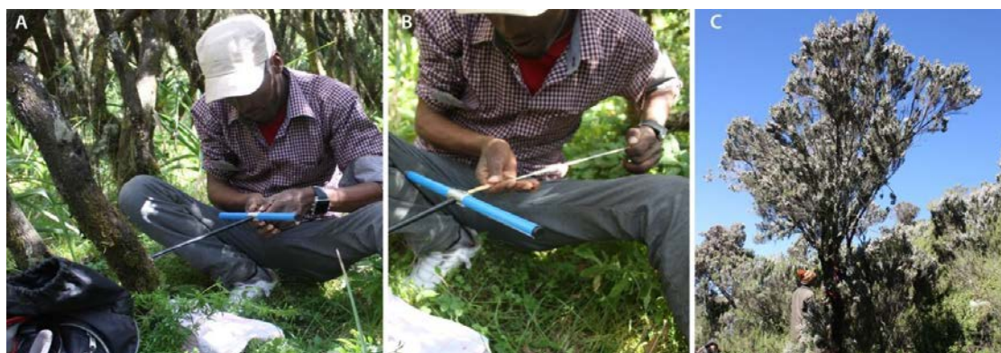
Figure 3. Wood sample collection using an increment borer in Lib Amba Mountain: (A,B) tree coring and core extraction; (C) Erica arborea tree at Lib Amba Mountain.
