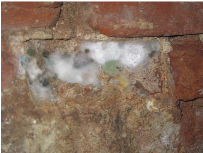
FIGURE 14 Detail of the zone a of Isabella Street, 4 weeks after the treatment with TEOS. A severe mould growth can be seen.
