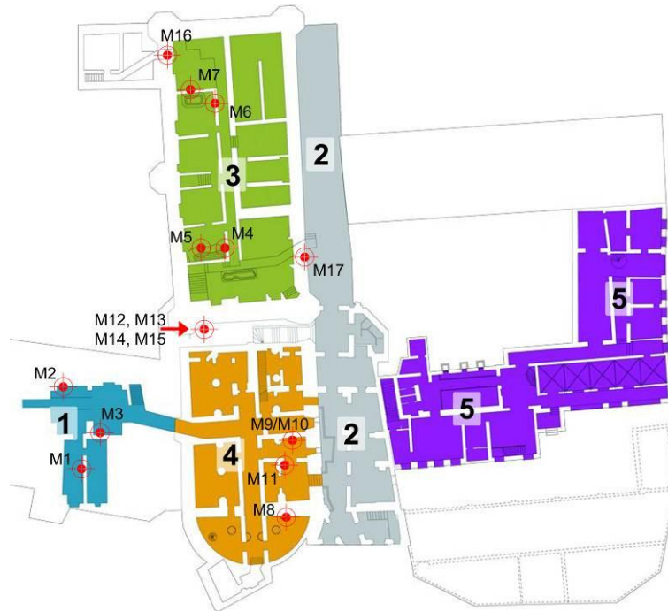
Figure 1: Plan overlaying the Coudenberg archaeological site and museum on the current Place Royale (Royal Square); 1. Main building, 2. Rue Isabelle (Isabella Street), 3. Aula Magna, 4. Chapel and 5. Hôtel d'Hoogstraeten (Hoogstraeten House). The location of the 17 mortar samples is marked on the plan. The samples M12 to M15 were lifted on the outer corner of the Aula Magna, almost at the level of the Royal Square (a level several meters above the underground archaeological site), where some remains of ancient dwellings pre-dating the construction of the Aula Magna have been discovered.
