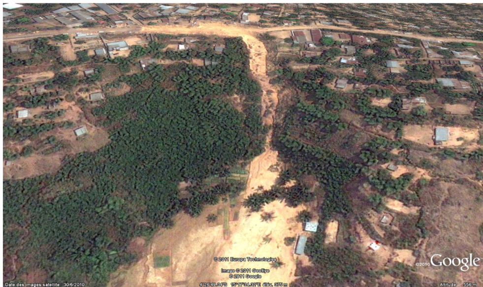
Fig. 4. New quickly developing leak mega-gully along the road of Kimwenza, 4 km south of UNIKIN (Fig. 1). Progressive erosion from the side of the road with already pronounced gully head. Regressive erosion on the road. GoogleEarth, 30/06/2010. The gully complex is only a few months old at the moment when the picture was taken.
