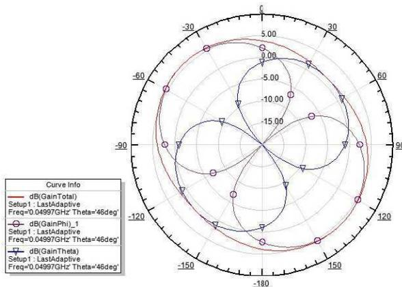
Figure 8 – Simulated gain in azimuth of a 3-element Yagi antenna pointing towards zenith (half of the cross-polarized antenna). The elevation is  $46^\circ$  from the ground.
