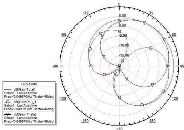
Figure 4 – Simulated gain in azimuth of a 3-element Yagi antenna tilted  $45^\circ$  in elevation and around its axis (half of the cross-polarized antenna). The elevation is  $46^\circ$  from the ground.
