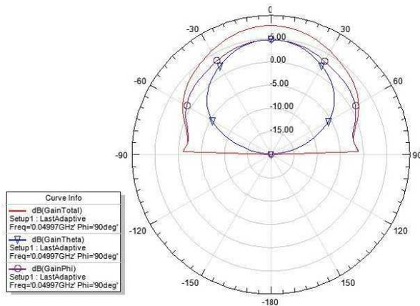
Figure 7 – Simulated gain in elevation of a 3-element Yagi antenna pointing towards zenith (half of the cross-polarized antenna). The azimuth is  $45^\circ$  from the E-plane.
