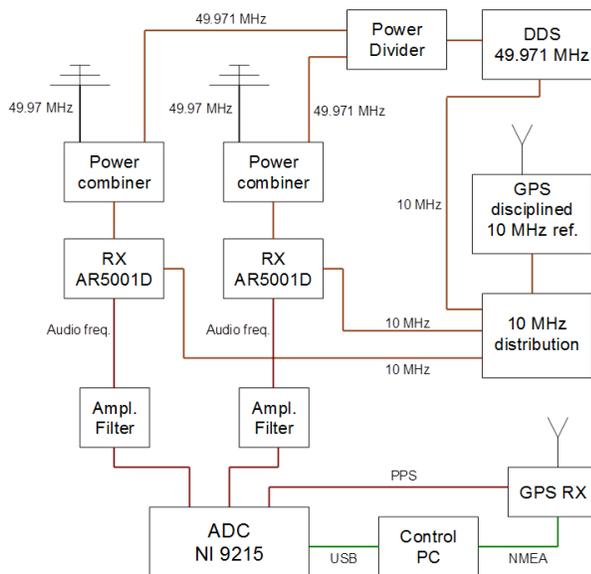
Figure 6 – Future measurement set-up.
