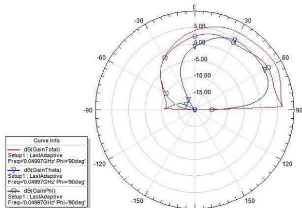
Figure 3 – Simulated gain in elevation of a 3-element Yagi antenna tilted  $45^\circ$  in elevation and around its axis (half of the cross-polarized antenna). The azimuth is  $45^\circ$  from the antenna boom.
