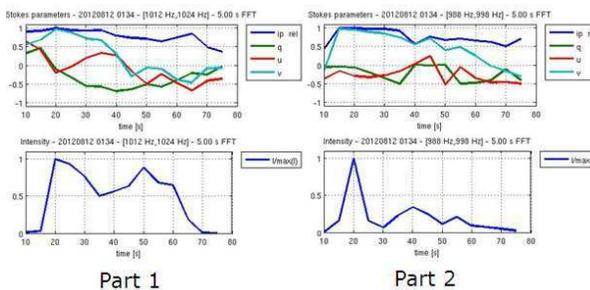
Figure 14 – Parameters  $I_p$ ,  $Q$ ,  $U$ ,  $V$ , and  $I/I_{\max}$  of echo MB1.
