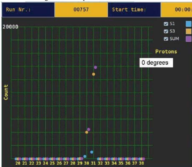
Fig. 2: Counts in the EPT channels for a 62 MeV proton beam at 0° incidence angle, at the UCL Light ions Irradiation Facility (LIF).
