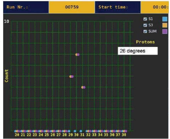
Fig. 3: Counts in the EPT channels for a 62 MeV proton beam at 26° incidence angle, at the UCL Light ions Irradiation Facility (LIF).
