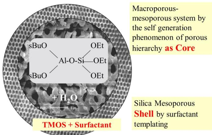
**Figure 32.** Synthesis strategy used for the fabrication of meso-macroporous core/highly ordered mesoporous shell structure
