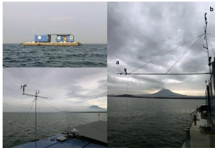
Figure 60: The EAGLES Automatic Weather Station on Lake Kivu after its installation, 8 October 2012 (© Wim Thiery).
