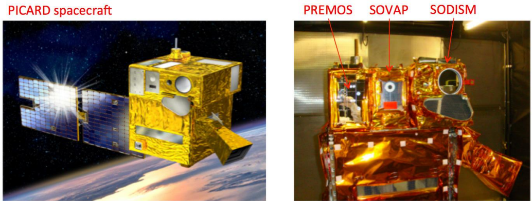
Figure 1: (left) Artist's view of the PICARD spacecraft. Credits: CNES - D. Ducros. (right) PICARD spacecraft with its scientific payload during integration phase in 2009.
