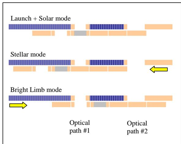
**Figure 15: Position of shutter mechanism during the different observation modes (the figure shows a cross section of satellite wall and shutter mechanism)**
