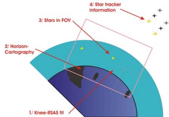
**Figure 2: Illustration of the ALTIUS concept. The attitude registration is performed by the combination of the star tracker information, the position of stars in FOV and geographic features**
