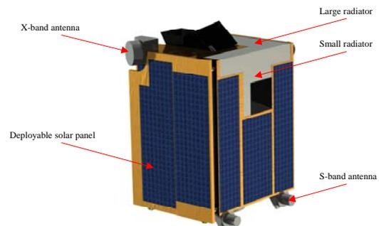
Figure 5: External accommodation with solar panel in stowed configuration
