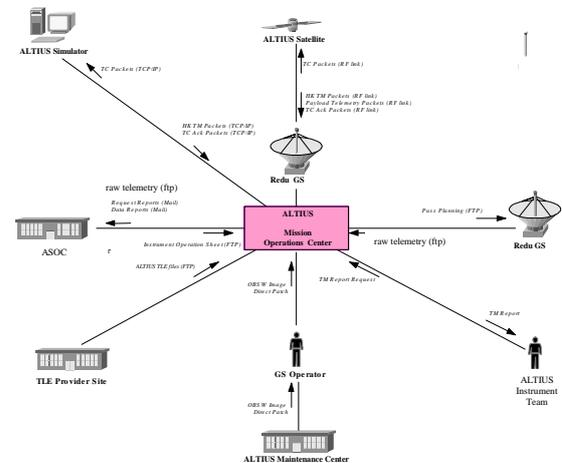
Figure 18: Interfaces to external systems seen from the AMOC
