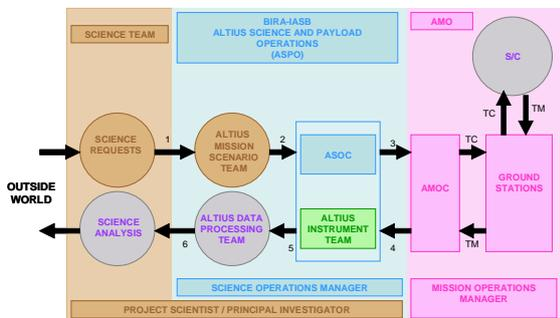
Figure 16: General structure of the ALTIUS ground segment
