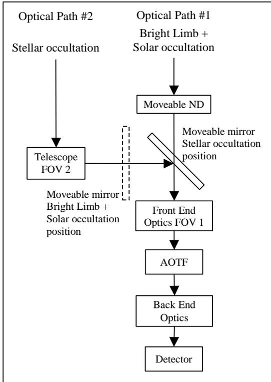
**Figure 10: Schematic representation of the optical layout of the instrument**
