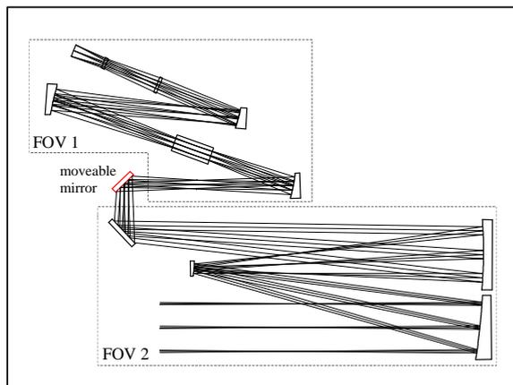
**Figure 12: Conceptual optical design of visible channel with the moveable mirror (red) in the stellar occultation position.**
