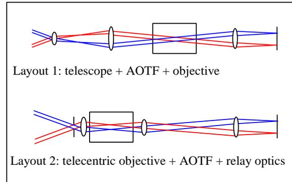
**Figure 11: Schematic layouts for ALTIUS**
