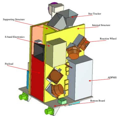
Figure 4: Internal accommodation of the ALTIUS spacecraft
