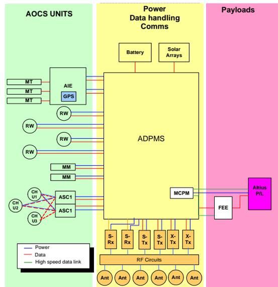
Figure 6: ALTIUS S/C electrical architecture
