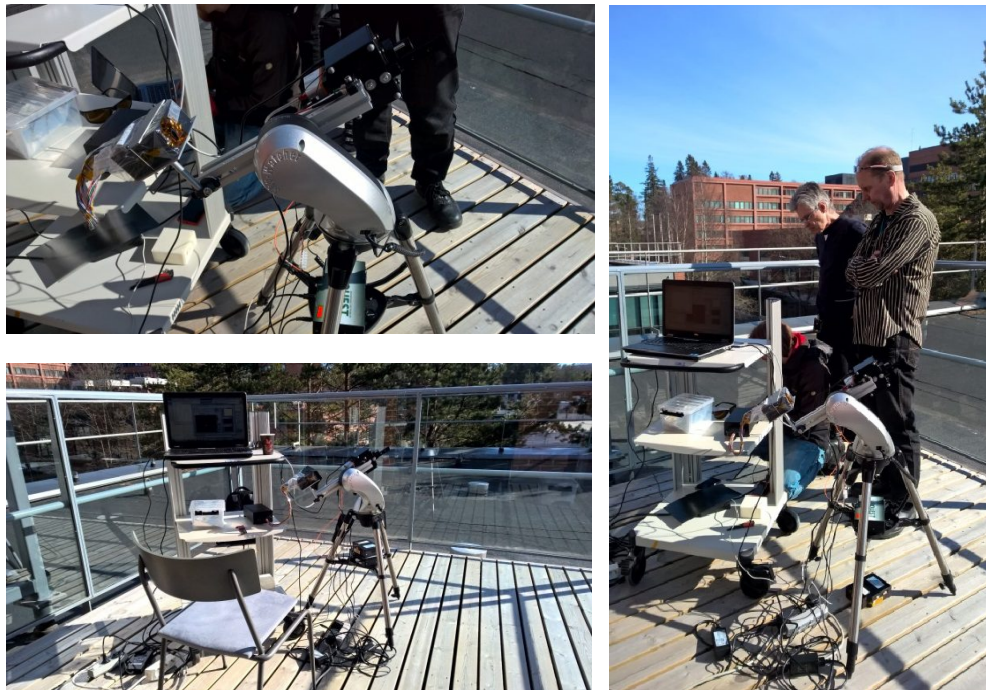
Figure 18. Measurement setup for the ground based measurements. VISION-EM (the camera at the rear) and a SWIR spectral camera (the camera at the front) are attached to the tripod. Reference spectrometer for the SWIR camera is also visible (Ocean Optics NIR-Quest).
