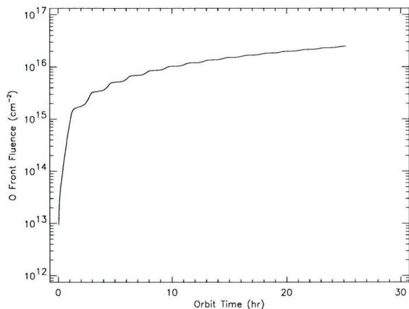
Figure 15. MSISE-90 Atomic oxygen fluence on a plate perpendicular to the spacecraft velocity vector for an 800 km heliosynchronous orbit
