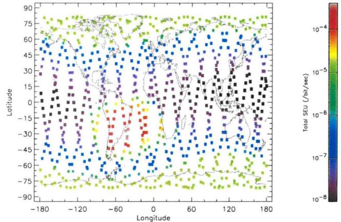
Figure 5. Single event upset rates along an 800 km heliosynchronous orbit
