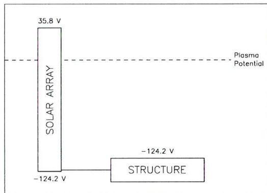
Figure 16. SOLARC Solar array/structure grounding configuration
