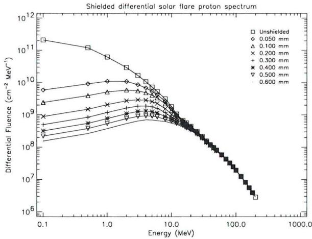
Figure 6. Shielded differential solar proton spectrum for an 800 km heliosynchronous orbit
