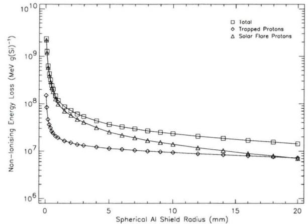
Figure 4. Non-ionising energy loss as a function of Al shield radius for an 800 km heliosynchronous orbit
