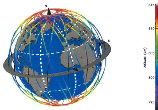
Figure 1. Three dimensional representation of an 800 km heliosynchronous orbit
