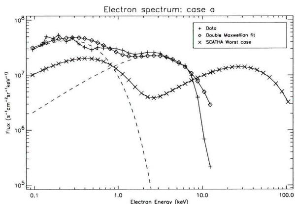
Figure 17. Double Maxwellian fit to a Gorizont/ADIPE electron charging event spectrum
