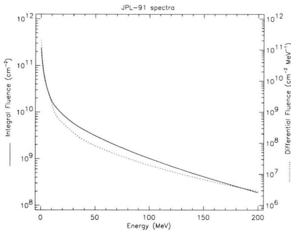
Figure 2. Integral and differential solar proton spectrum for an 800 km heliosynchronous orbit
