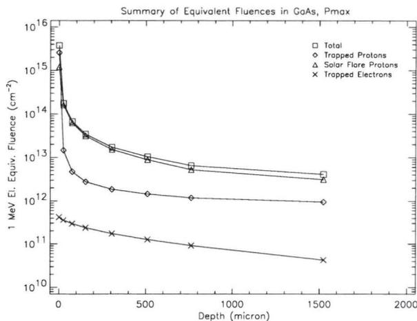
Figure 3. Equivalent fluences in a GaAs solar cell for an 800 km heliosynchronous orbit
