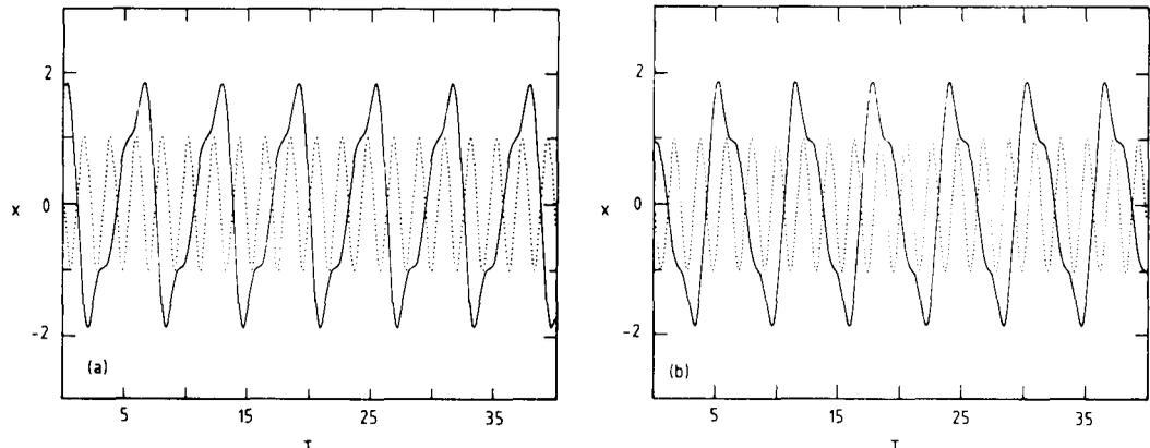
Fig. 6. Time dependence of variable  $x$  of the 2 period-3 solutions ((a) and (b)) for the same parameter values as in Fig. 4 but with  $q = 13.5q_c$ . The dotted line represents the forcing with amplitude normalized to unity. Notice that the 2 solutions exhibit different phase-shifts relative to the forcing.
