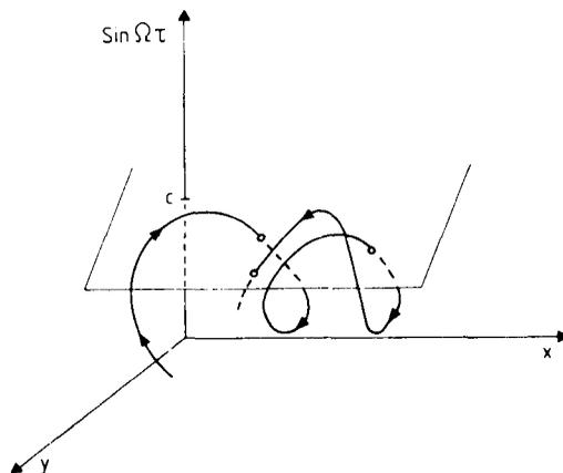
Fig. 3. Schematic representation of a Poincaré map for a forced system. As the system evolves, a representative trajectory cuts a plane of section  $C$  at discrete times  $\tau_n$ . The study of the dynamics on the surface of the section gives valuable information on the qualitative behavior of the initial system.
