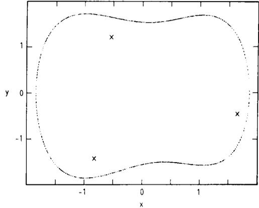
Fig. 4. Poincaré map of the forced system eqs. (8) for  $\gamma_2 = 1$ ,  $\gamma_1 = 1.01$ ,  $\mu = 0.1$ ,  $\Omega = 3$  and  $q = q_c + 0.2$ , where  $q_c = 1.96$ . Depending on the initial conditions, the system evolves either to a quasi-periodic attractor (closed curve) or to a periodic one, with a period 3 times as large as the forcing period (points and crosses).
