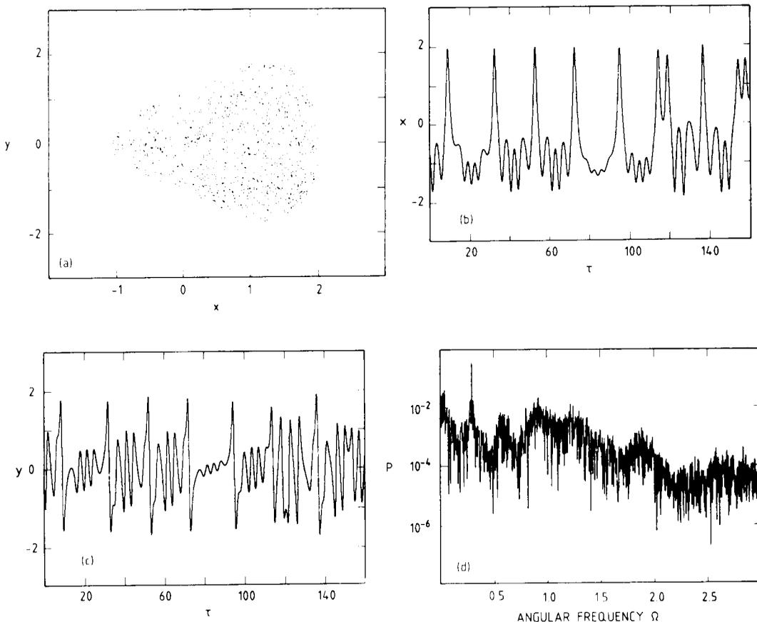
Fig. 8. Numerical integration of eqs. (8) for the same parameter values as in Fig. 4 but  $\Omega = 0.3$  and  $q = 50q_c$ , where now  $q_c = 0.148$ . (a) Poincaré map; (b) time evolution of variable  $x$ ; (c) time evolution of variable  $y$ ; (d) power spectrum of variable  $x$ .
