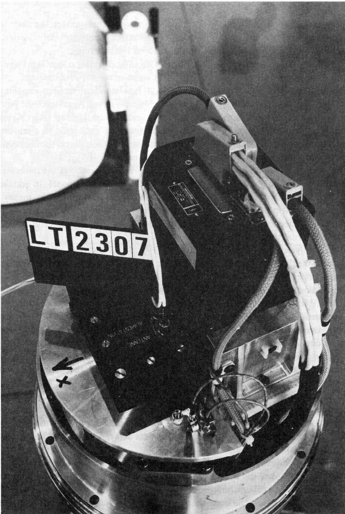
Fig. 4. Upper part of the NO-II payload, with nose cone removed, showing the upper plate with the radar transponder (left) and the security box (right). One of the Vibrachoc shock-mounts is partly visible below the upper plate.
