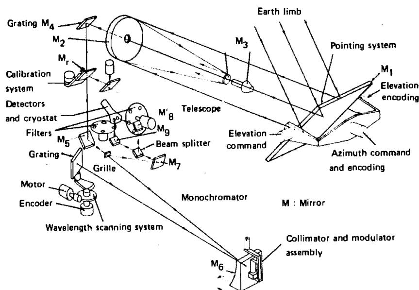
Fig. 2.- Optical diagram of the instrument. The characteristic parts of the grille spectrometer are the grille itself, used in transmission as entrance and in reflexion as exit slit and the vibrating parabolic mirror  $M_6$  which aligns the spectrometer once in each oscillation, defining a built in modulation.
