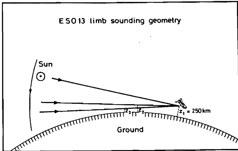
Fig. 1.- Observational geometry during a sunset. The spacecraft being at an altitude of 250 km, the spectrometer heliostat follows the sun as it goes down. At zenith angles greater than 90 degrees, the altitudes  $z_2$  and  $z_3$  where the rays are the closest to the earth surface are the zones of main absorption and will be referred as the altitudes of the observation.
