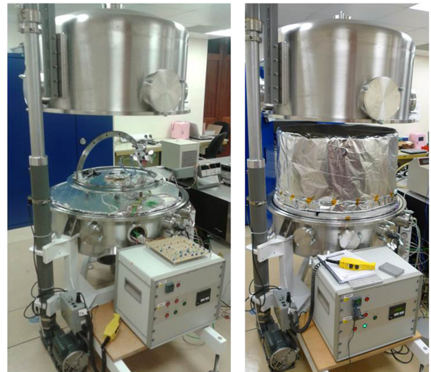
FIG. 8. Photographs showing thermal infrared setup. (Left) The OSEG setup inside the vacuum chamber without the cold shield surrounding it. (Right) The cold shield surrounded by 10 layers of multilayer insulation (MLI) house inside the vacuum chamber.
