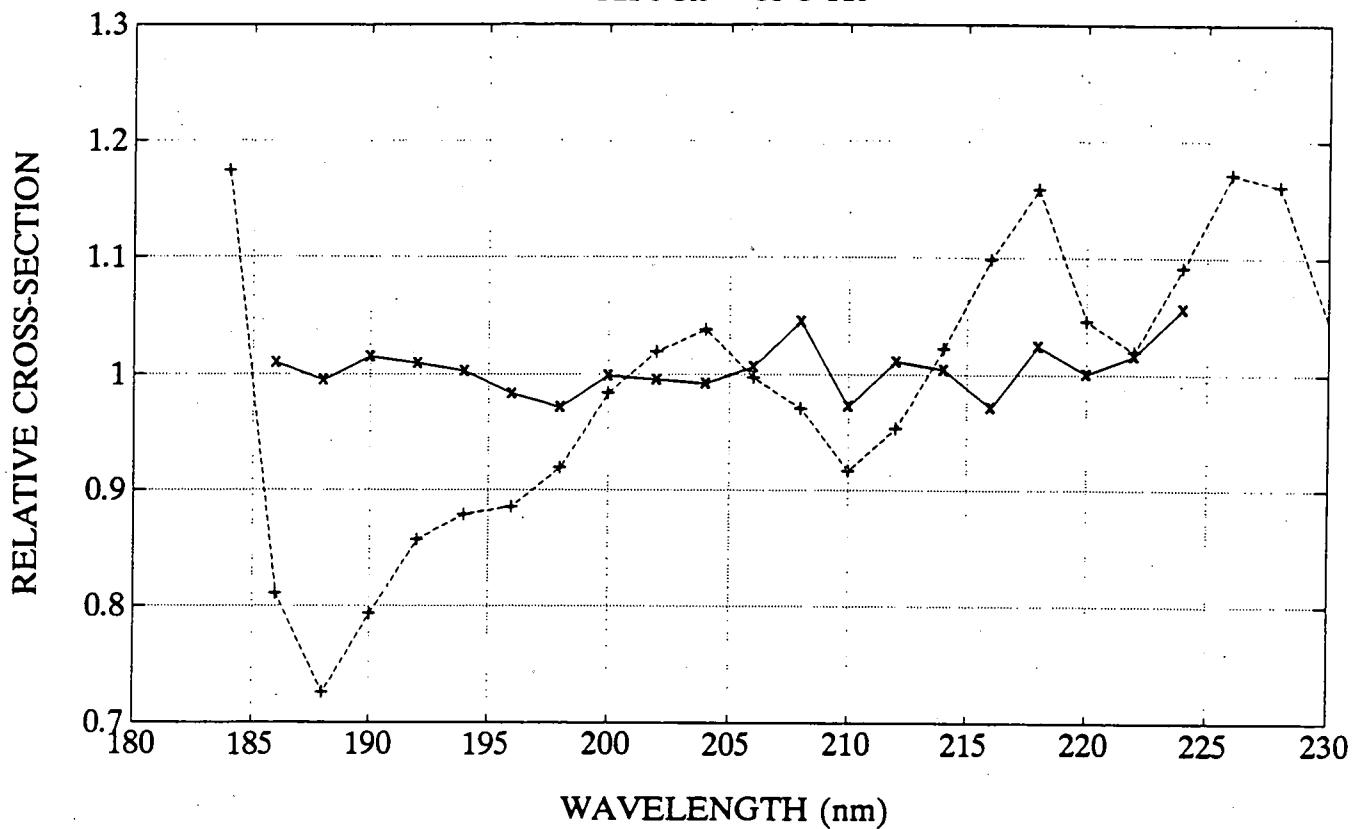
Figure 18. Relative absorption cross-sections of C<sub>2</sub>F<sub>3</sub>Cl<sub>3</sub> at room temperature, as a function of wavelength.
