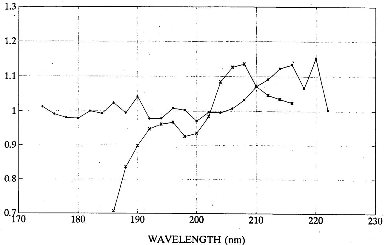
Figure 13. Relative absorption cross-sections of CHFC<sub>2</sub> at room temperature, as a function of wavelength.
