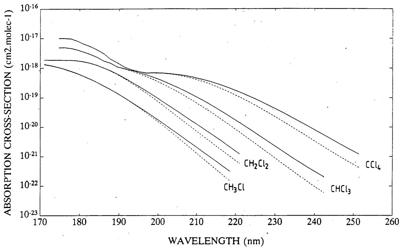
Figure 2. U.V. Absorption cross-sections of chloromethanes as a function of wavelength.
