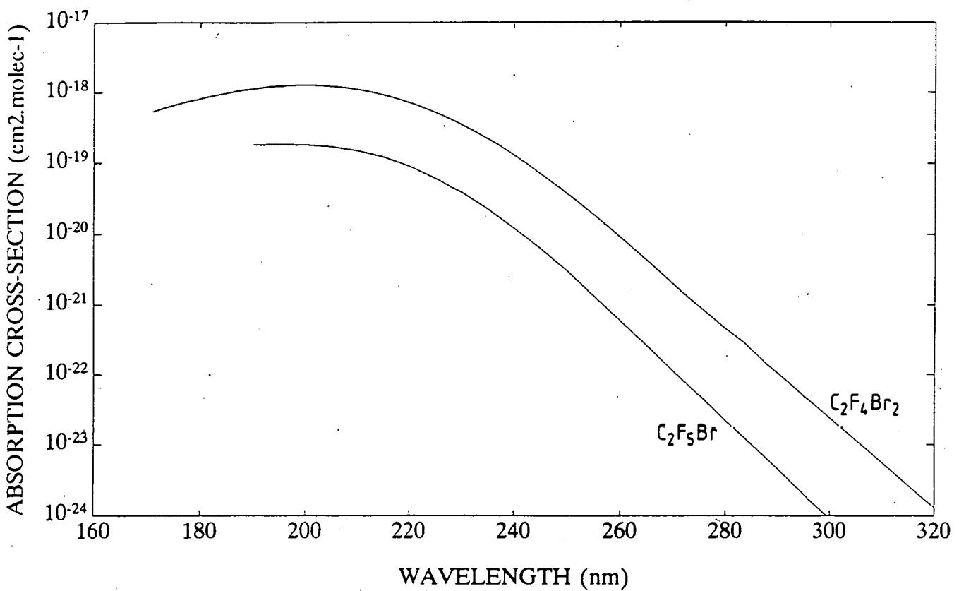
Figure 26. U.V. Absorption cross-sections of bromoethanes as a function of wavelength.
