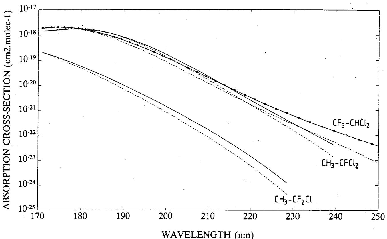
Figure 15. U.V. Absorption cross-sections of hydrochlorofluoroethanes as a function of wavelength.
