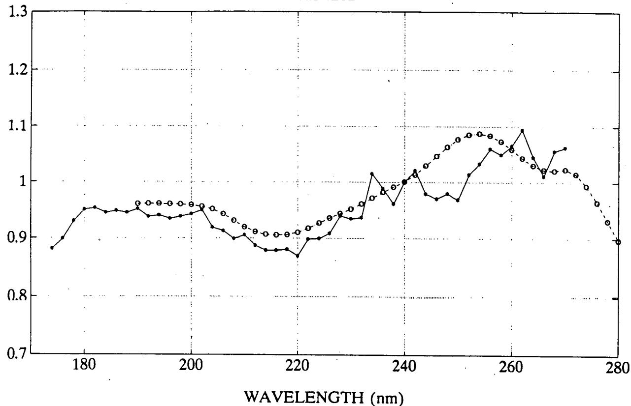
Figure 32. Relative absorption cross-sections of C<sub>2</sub>F<sub>4</sub>Br<sub>2</sub> at room temperature, as a function of wavelength.
