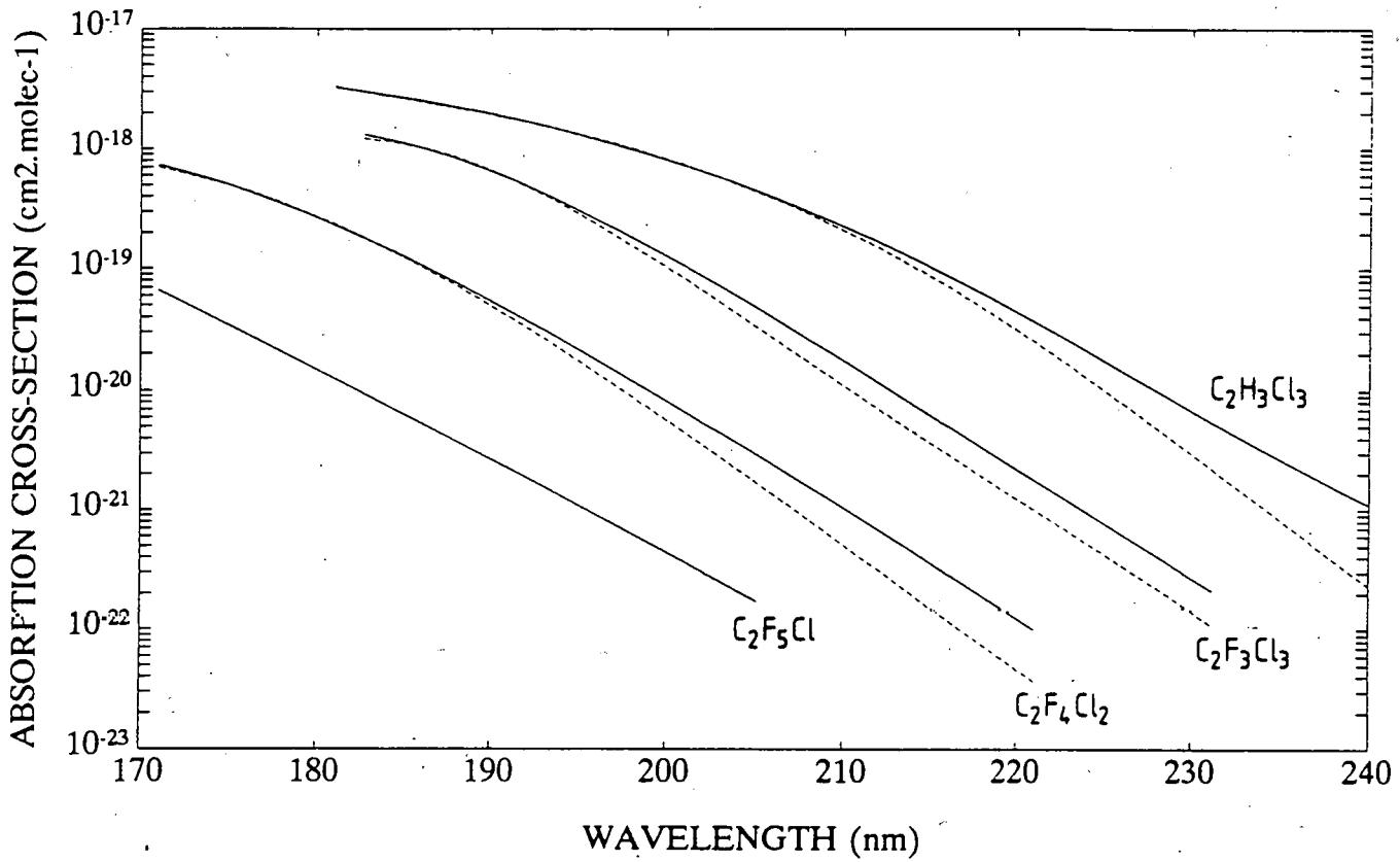
Figure 14. U.V. Absorption cross-sections of chloro- and chlorofluoroethanes as a function of wavelength.
