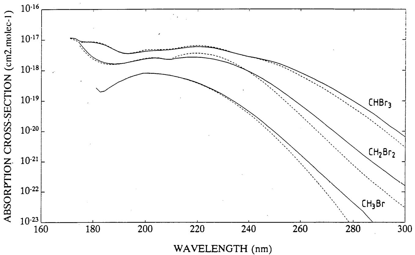
Figure 24. U.V. Absorption cross-sections of bromomethanes as a function of wavelength.
