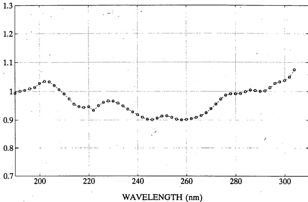
Figure 30. Relative absorption cross-sections of  $\text{CF}_2\text{Br}_2$  at room temperature, as a function of wavelength.
