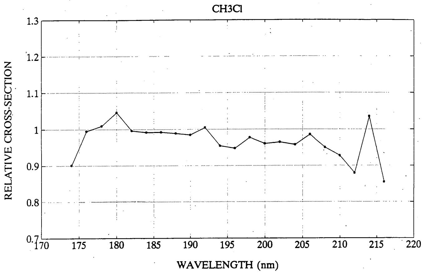
Figure 5. Relative absorption cross-sections of CH<sub>3</sub>Cl at room temperature, as a function of wavelength.
