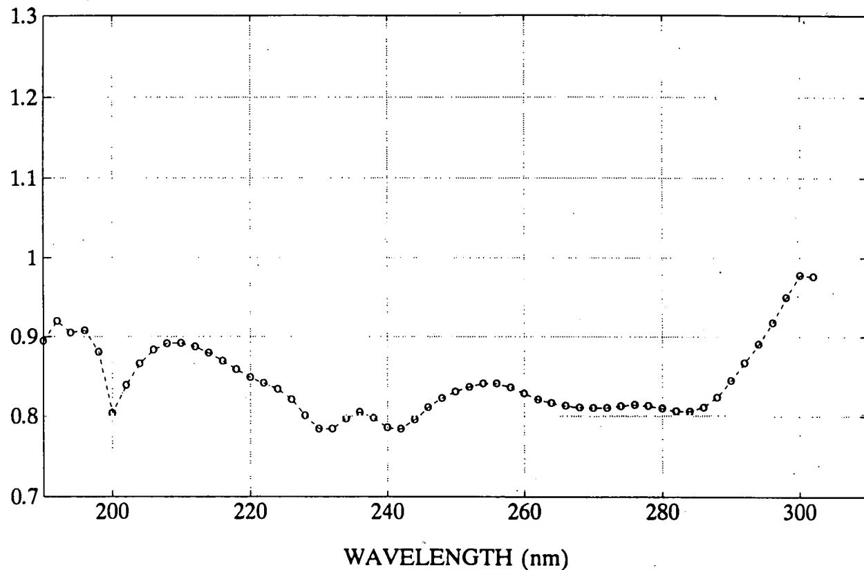
Figure 31. Relative absorption cross-sections of  $\text{CF}_2\text{BrCl}$  at room temperature, as a function of wavelength.
