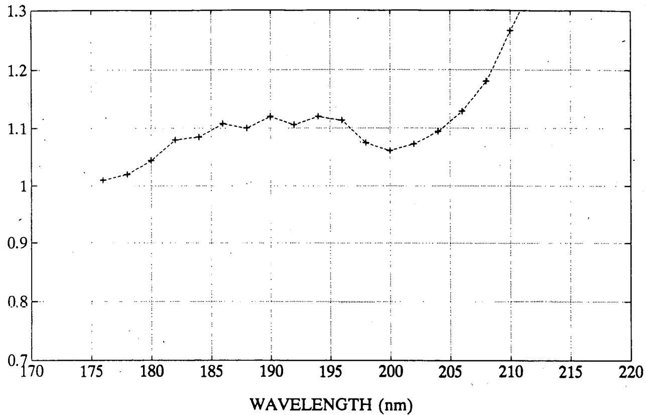
Figure 6. Relative absorption cross-sections of  $\text{CH}_2\text{Cl}_2$  at room temperature, as a function of wavelength.
