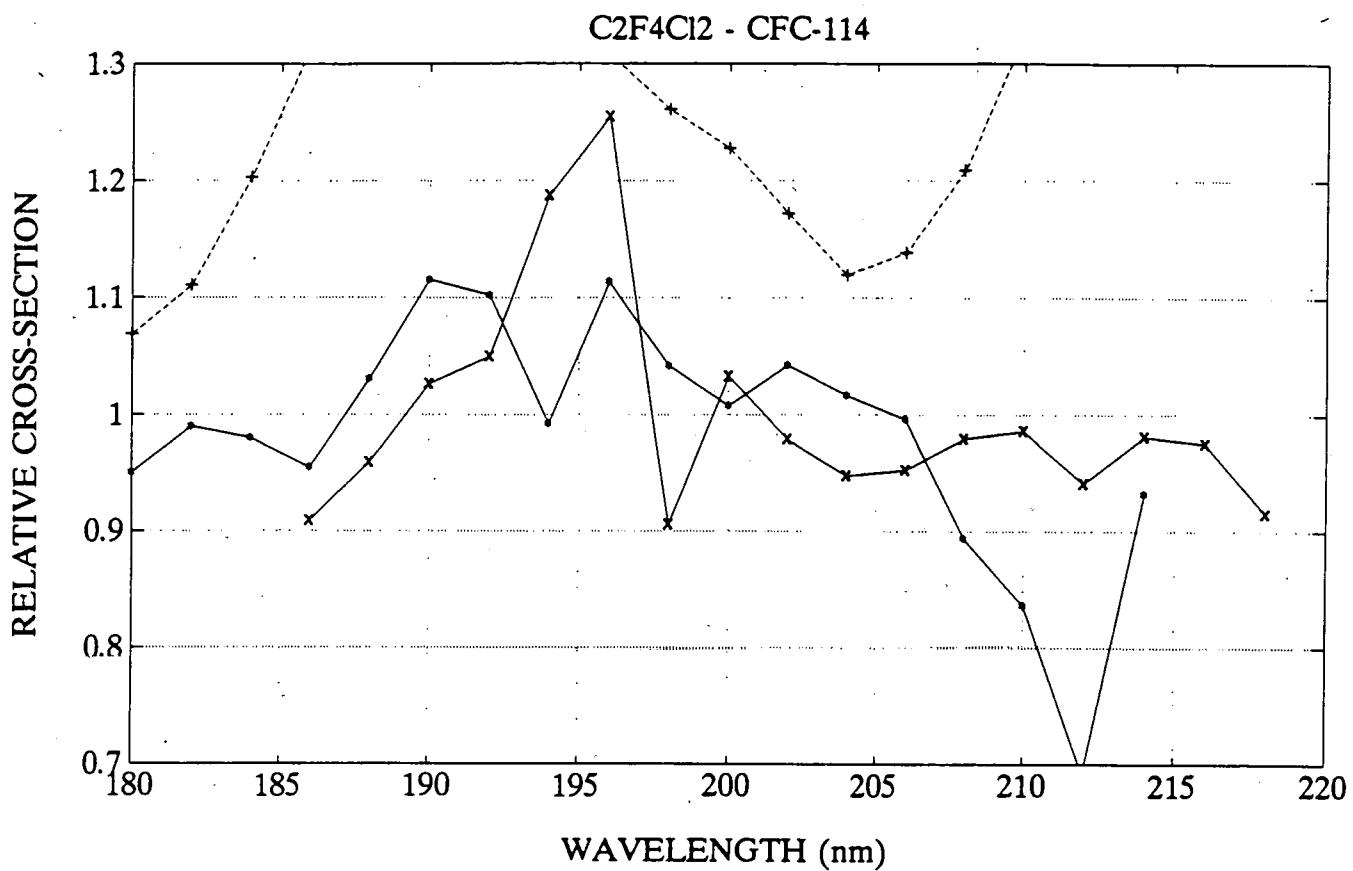
Figure 19. Relative absorption cross-sections of C<sub>2</sub>F<sub>4</sub>Cl<sub>2</sub> at room temperature, as a function of wavelength.
