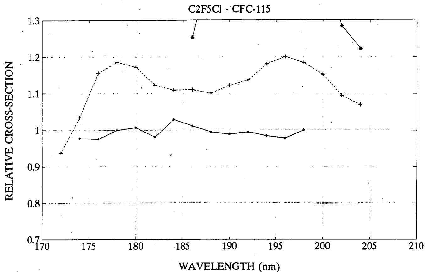
Figure 20. Relative absorption cross-sections of C<sub>2</sub>F<sub>5</sub>Cl at room temperature, as a function of wavelength.
