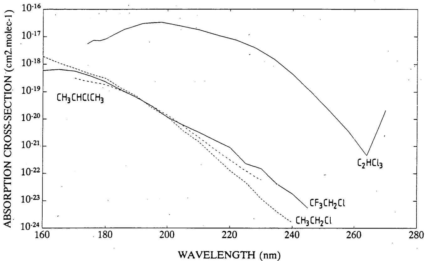
Figure 16. U.V. Absorption cross-sections of chlorofluoroethanes, chloroethylenes and chloropropane at ambient temperature as a function of wavelength.
