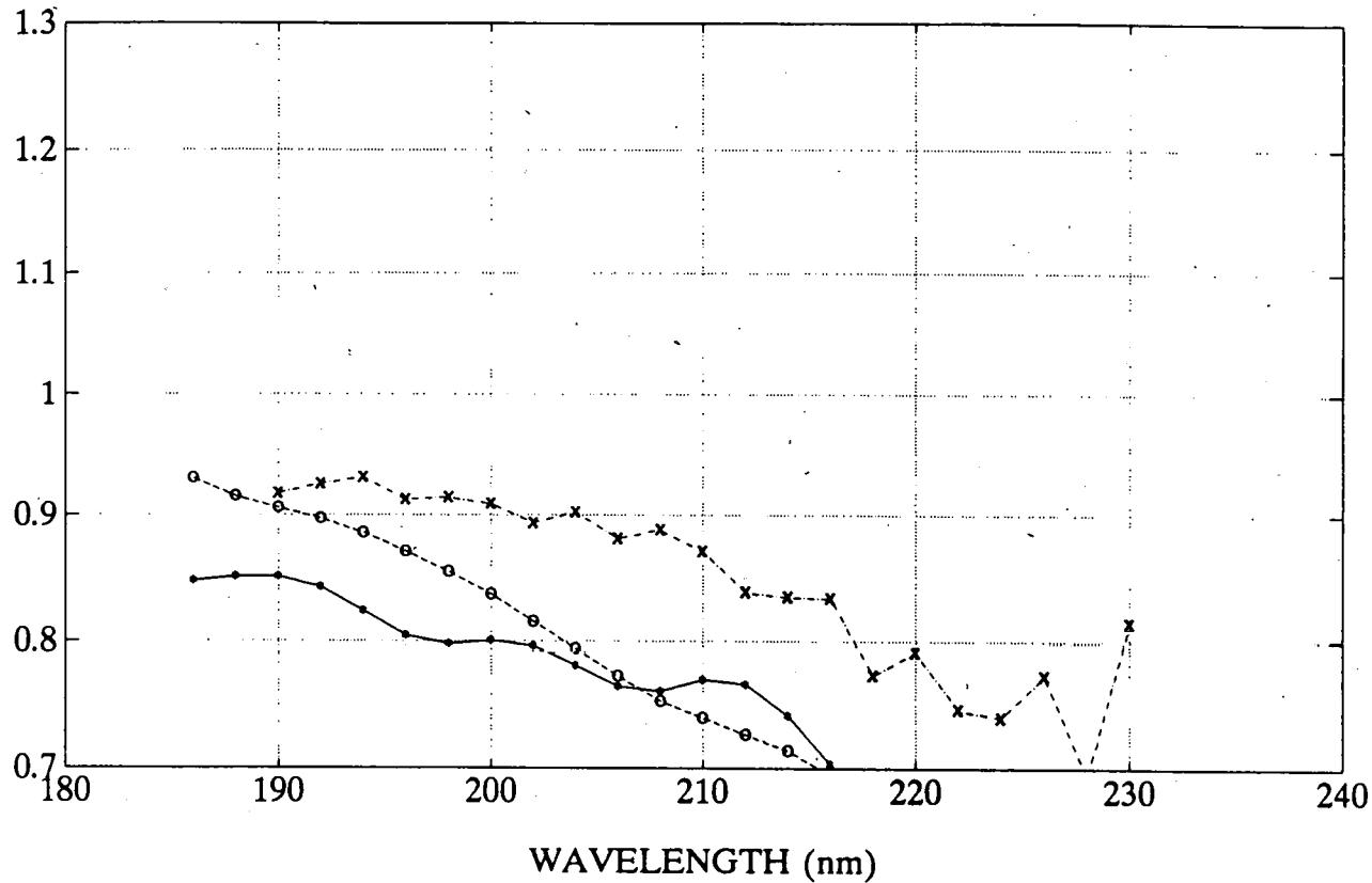
Figure 21. Relative absorption cross-sections of CF<sub>3</sub>-CHCl<sub>2</sub> at room temperature, as a function of wavelength.
