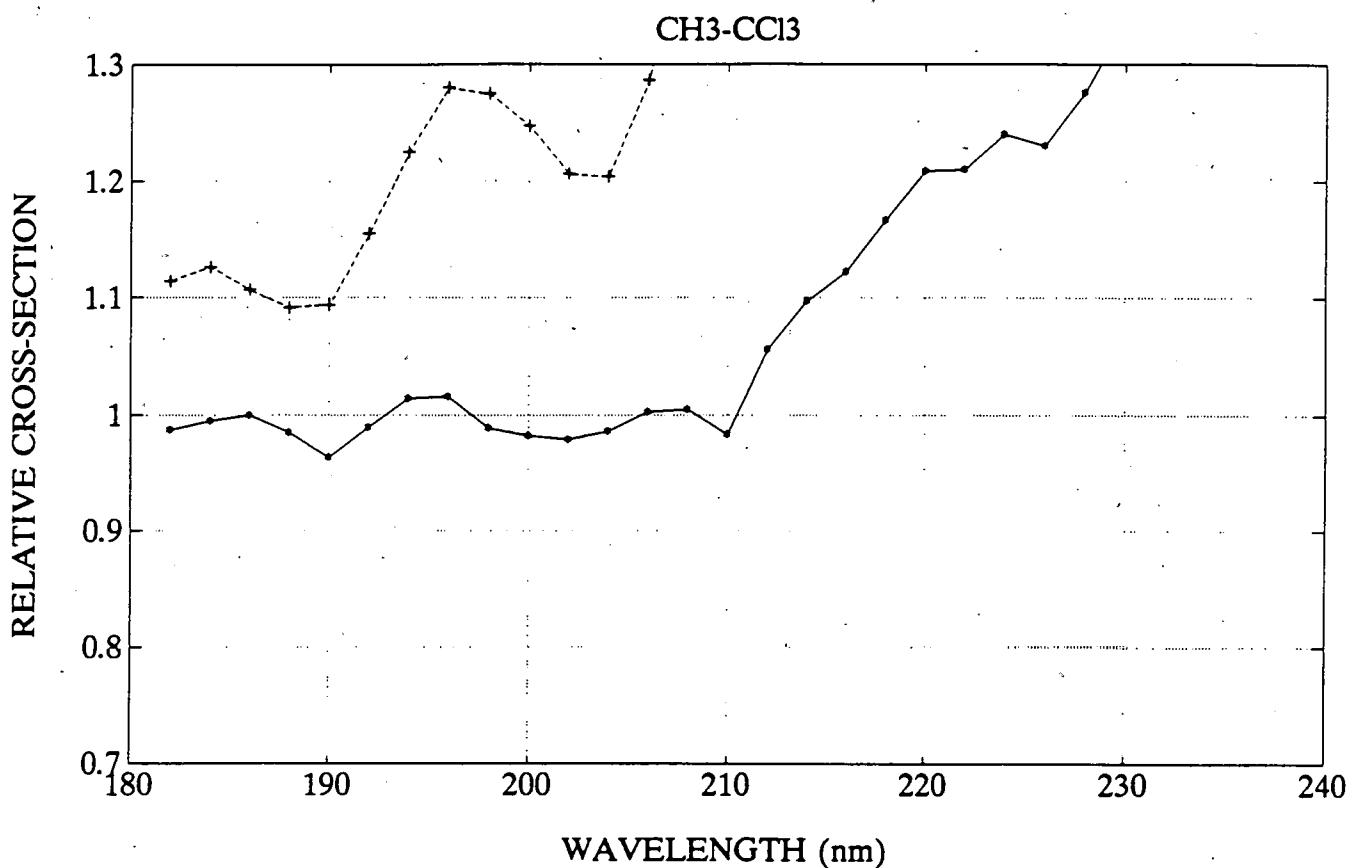
Figure 17. Relative absorption cross-sections of CH<sub>3</sub>-CCl<sub>3</sub> at room temperature, as a function of wavelength.
