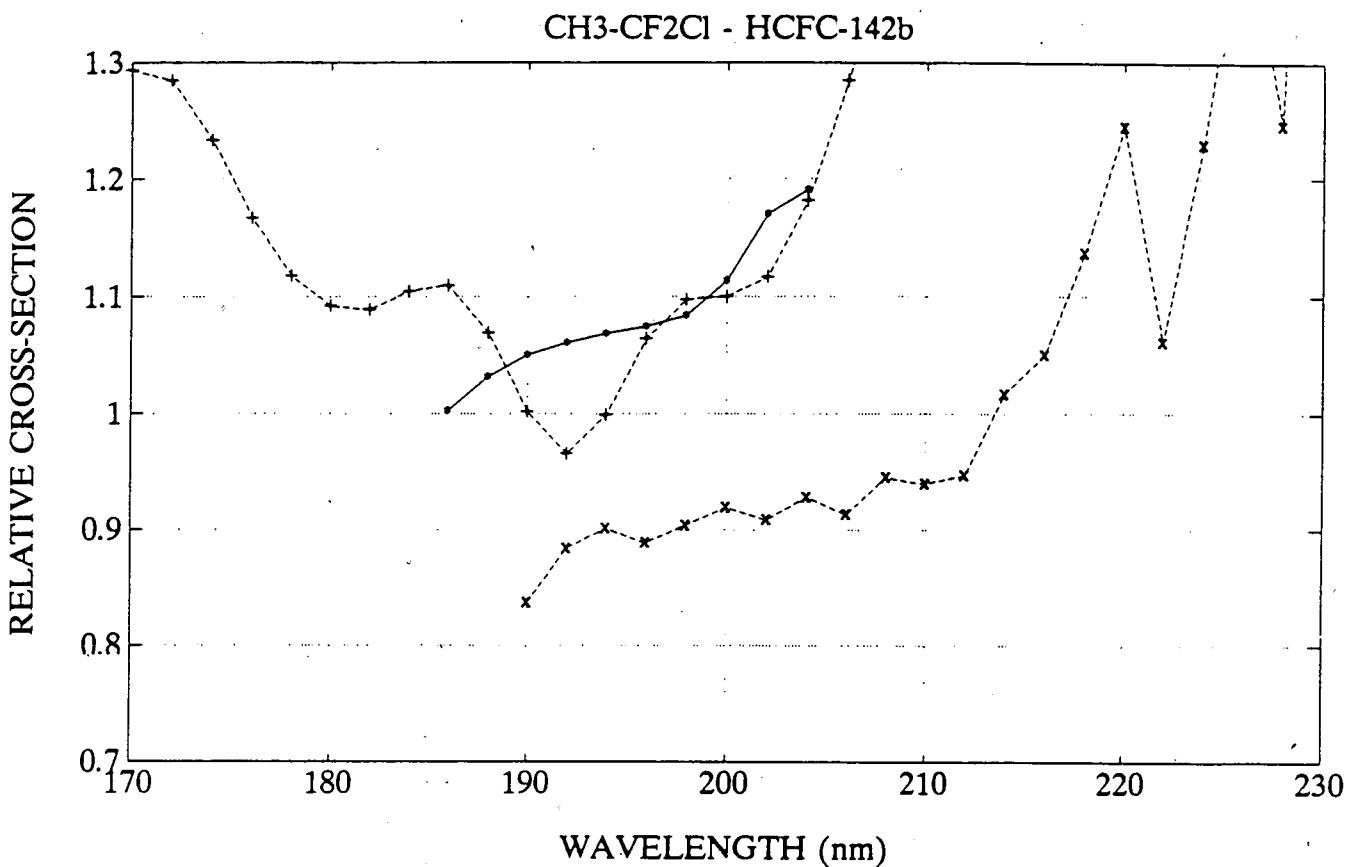
Figure 23. Relative absorption cross-sections of CH<sub>3</sub>-CF<sub>2</sub>Cl at room temperature, as a function of wavelength.
