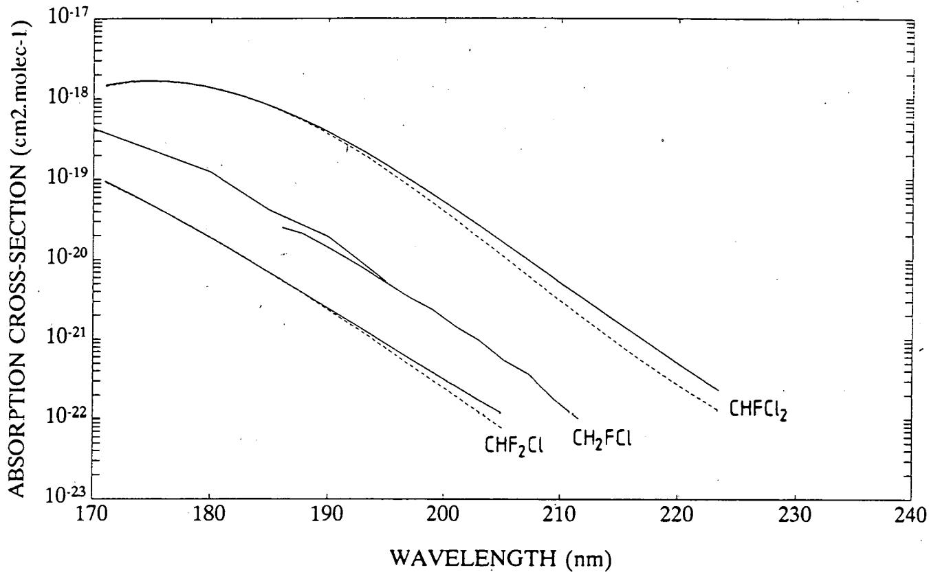
Figure 4. U.V. Absorption cross-sections of hydrochlorofluoromethanes as a function of wavelength.
