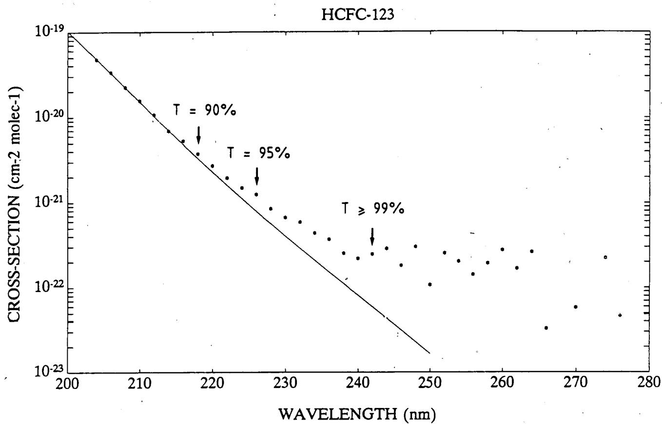
Figure 1. Comparison between cross-section values obtained for one pressure condition with unlimited range of transmitted flux (\*), and for various pressure conditions considering limited range of transmitted fluxes (—).
