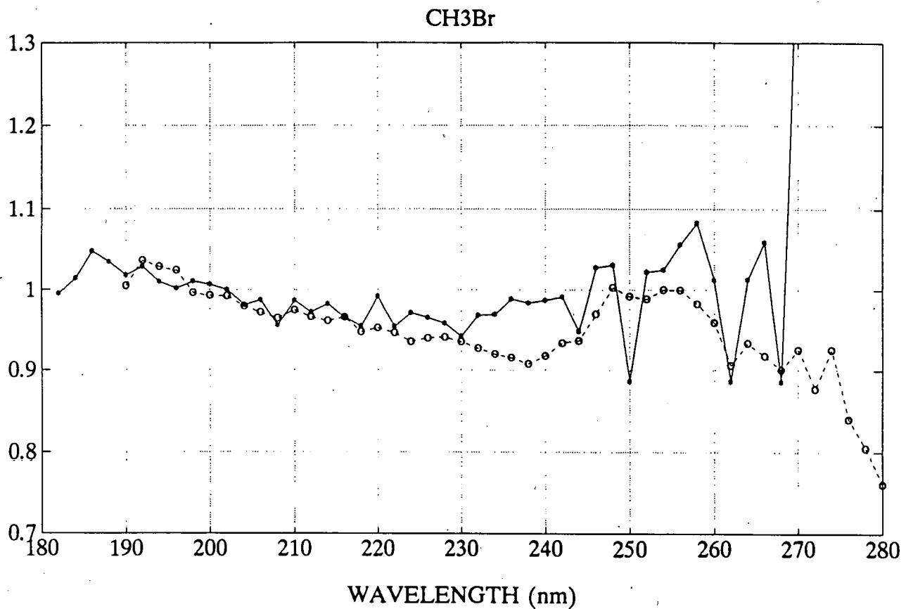
Figure 27. Relative absorption cross-sections of CH<sub>3</sub>Br at room temperature, as a function of wavelength.
