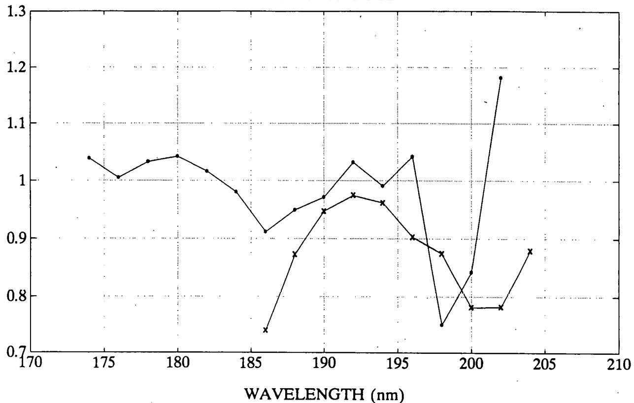
Figure 12. Relative absorption cross-sections of CHF<sub>2</sub>Cl at room temperature, as a function of wavelength.
