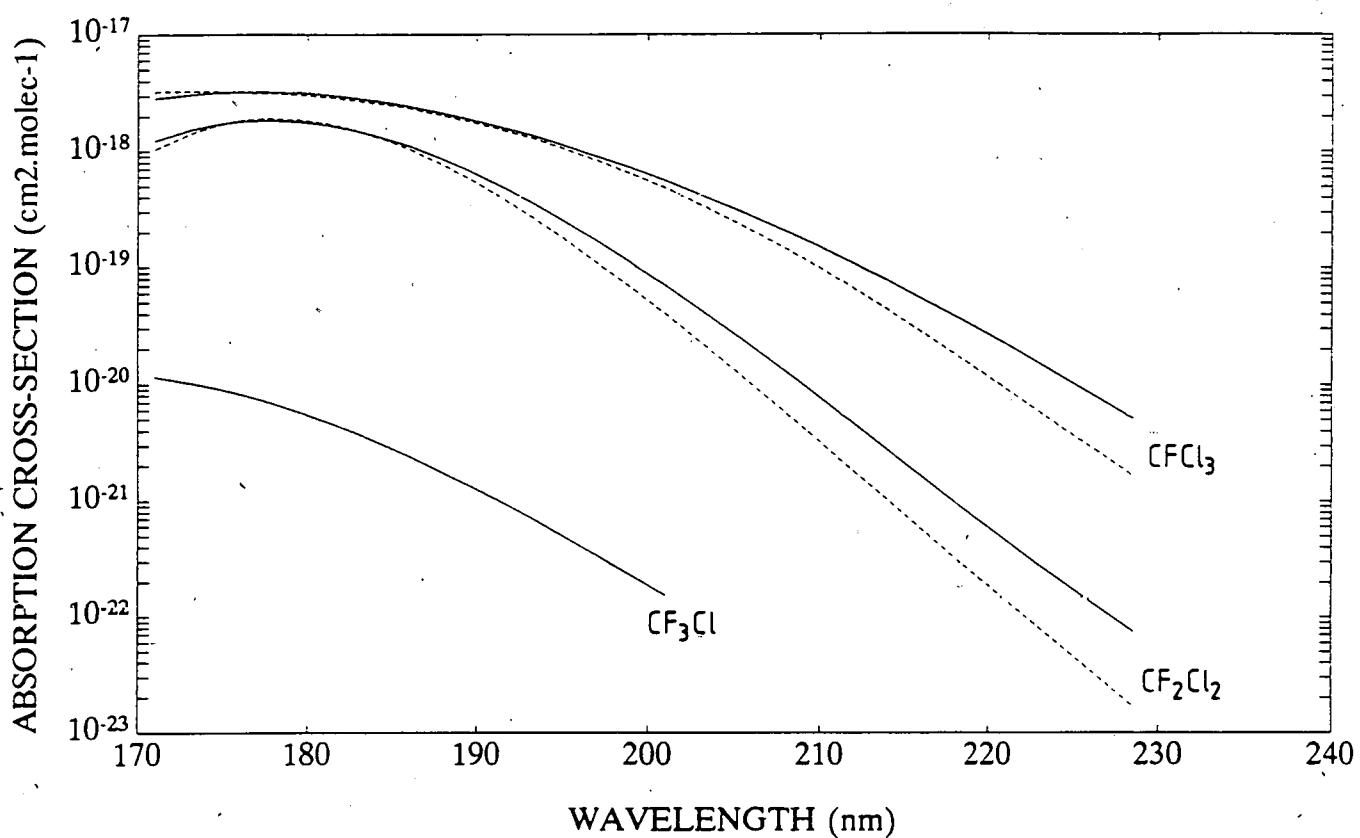
Figure 3. U.V. Absorption cross-sections of chlorofluoromethanes as a function of wavelength.
