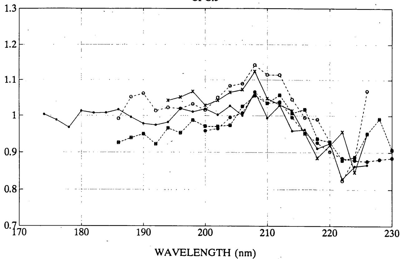
Figure 11. Relative absorption cross-sections of CFC<sub>3</sub> at room temperature, as a function of wavelength.
