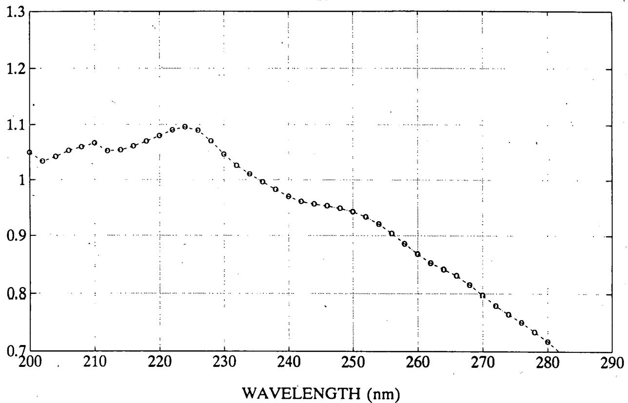
Figure 28. Relative absorption cross-sections of  $\text{CH}_2\text{Br}_2$  at room temperature, as a function of wavelength.
