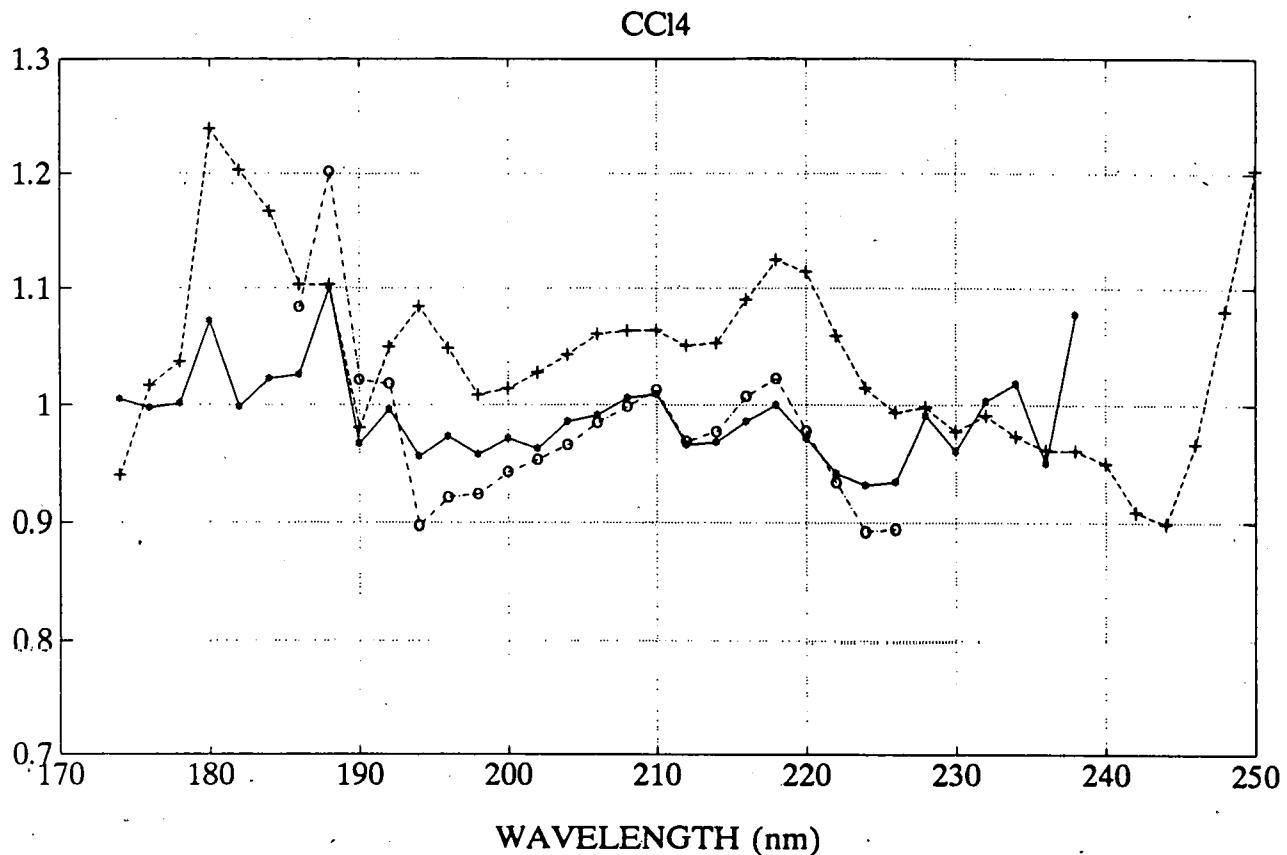
Figure 8. Relative absorption cross-sections of CCl<sub>4</sub> at room temperature, as a function of wavelength.
