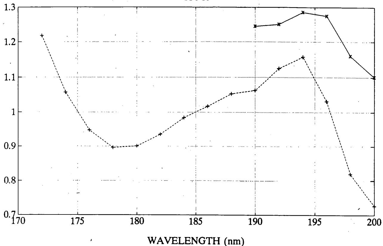
Figure 9. Relative absorption cross-sections of CF<sub>3</sub>Cl at room temperature, as a function of wavelength.
