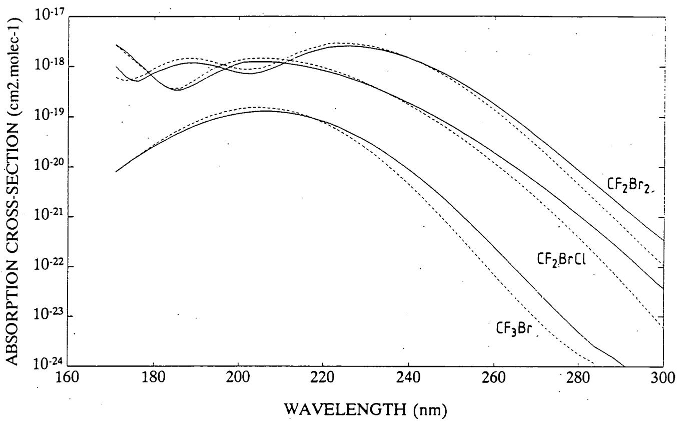
Figure 25. U.V. Absorption cross-sections of bromofluoromethanes as a function of wavelength.
