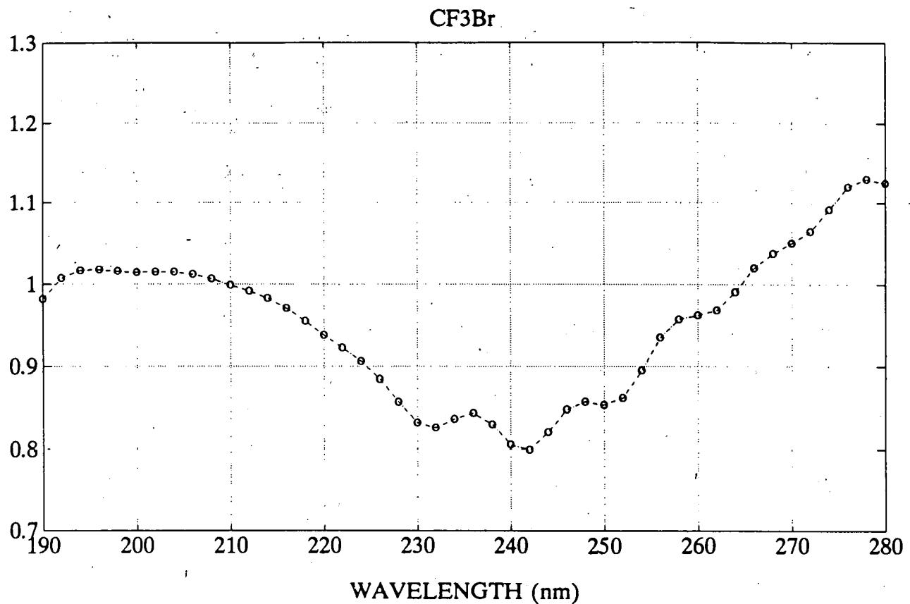
Figure 29. Relative absorption cross-sections of CF<sub>3</sub>Br at room temperature, as a function of wavelength.
