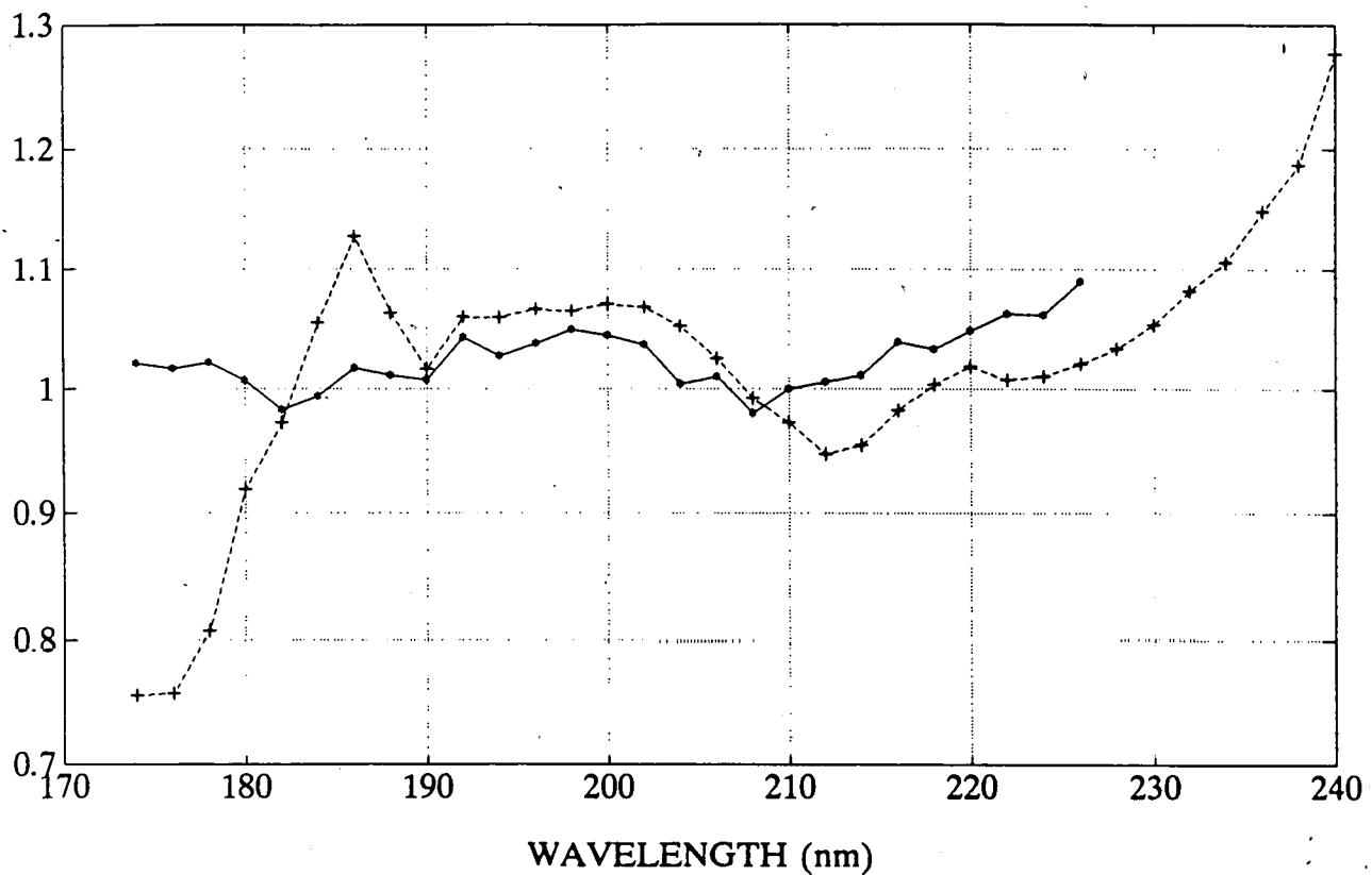
Figure 7. Relative absorption cross-sections of CHCl<sub>3</sub> at room temperature, as a function of wavelength.
