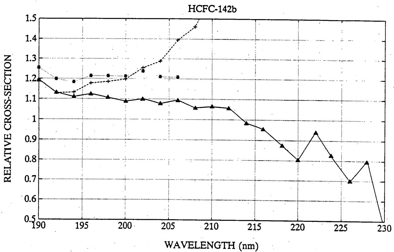
Figure 4. : Relative absorption cross-sections of HCFC-142b.
