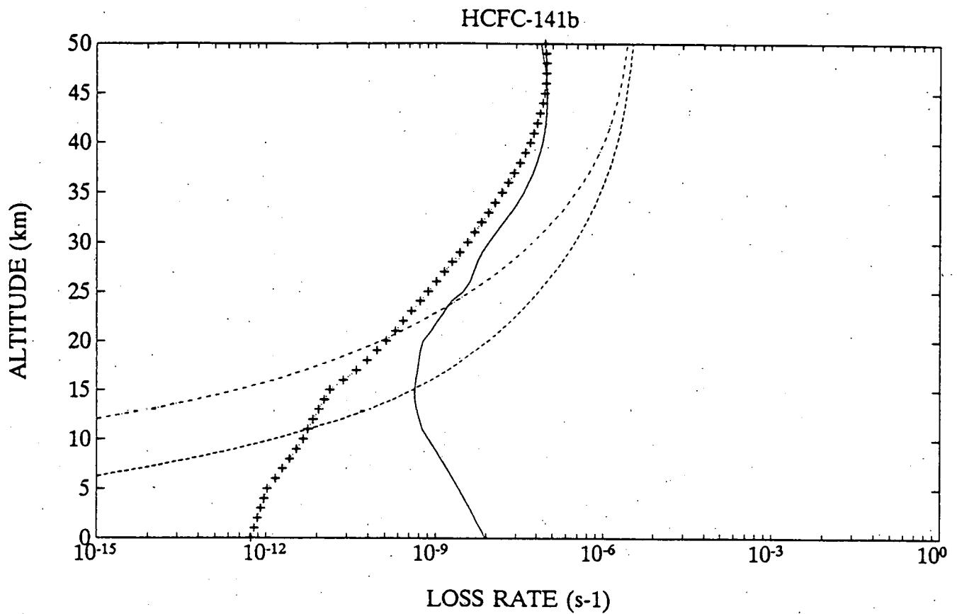
Figure 9. : Loss rates versus altitude for HCFC-141b.
