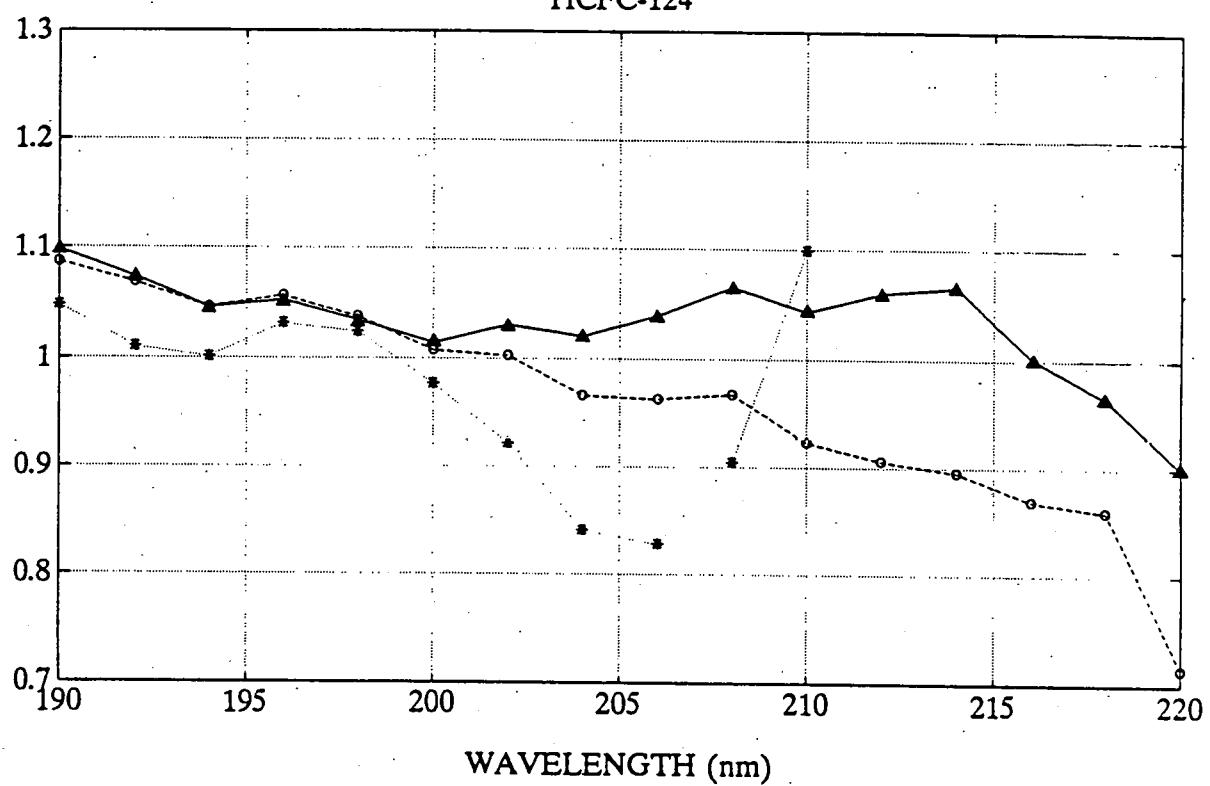
Figure 2. : Relative absorption cross-sections of HCFC-124.
