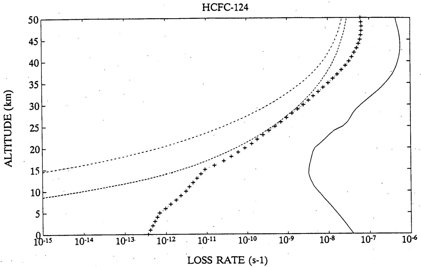
Figure 8. : Loss rates versus altitude for HCFC-124.
