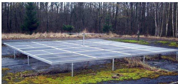
Figure 1 – BRAMS beacon radiating system in Dourbes, Belgium.
