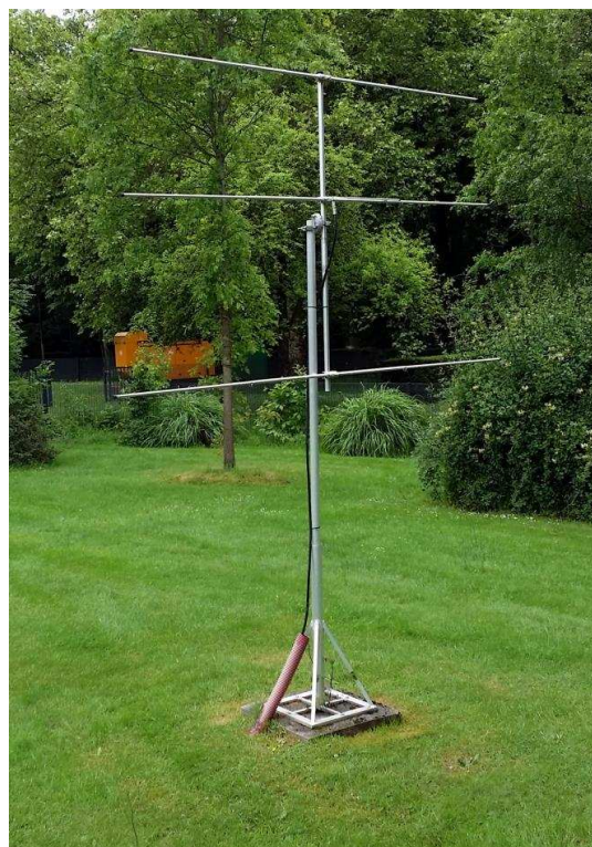
Figure 2 – Typical 3-element Yagi antenna of a BRAMS basic receiving system.
