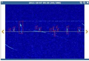
Figure 1 – A web application supports the manual counts of meteors in spectrograms. The horizontal axis represents the time (5 minutes in total), and the vertical axis the frequency (200 Hz centered on the horizontal line in the middle, which is the beacon). The user can interactively select regions of the spectrograms around possible meteor echoes and draw rectangles around them (indicated here as the red boxes). A distinction is made between short and long meteors.
