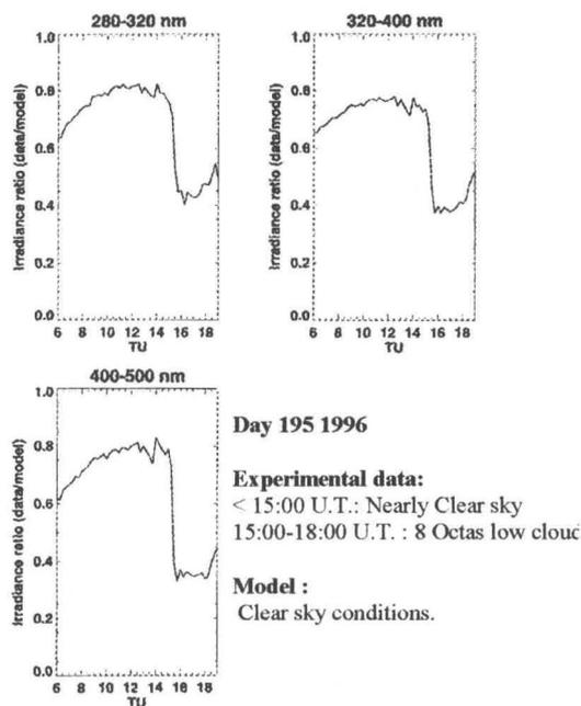
Figure 6. Ratio of measured to modelled irradiances.
