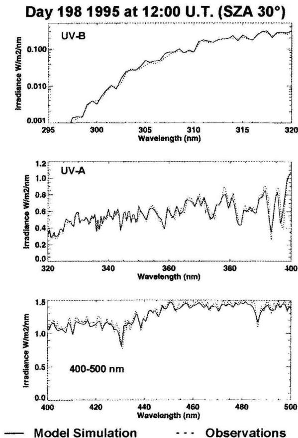
**Figure 3.** Comparison between experimental and modelled results for clear sky condition (Day 95-198).
