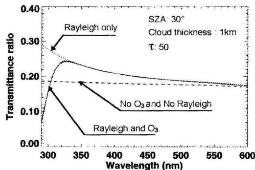
**Figure 5.** Simulated ratio of the mean clear sky spectrum vs. full cloud coverage.
