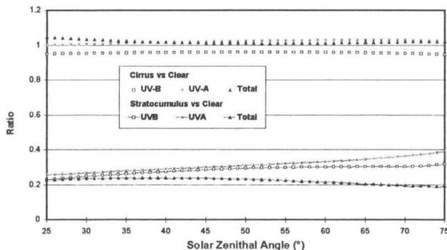
Figure 7. Irradiance ratio obtained from the pyranometers (Yearly average). Overcast sky (8 Octas) vs. clear sky.
