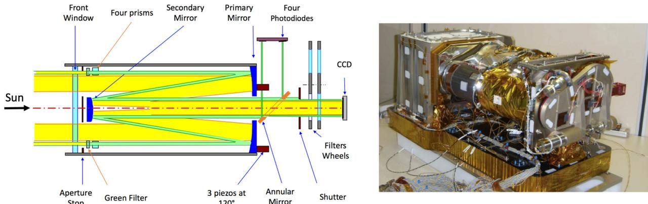
Figure 9: (left) PICARD/SODISM optical path. (right) The PICARD/SODISM instrument during integration.
