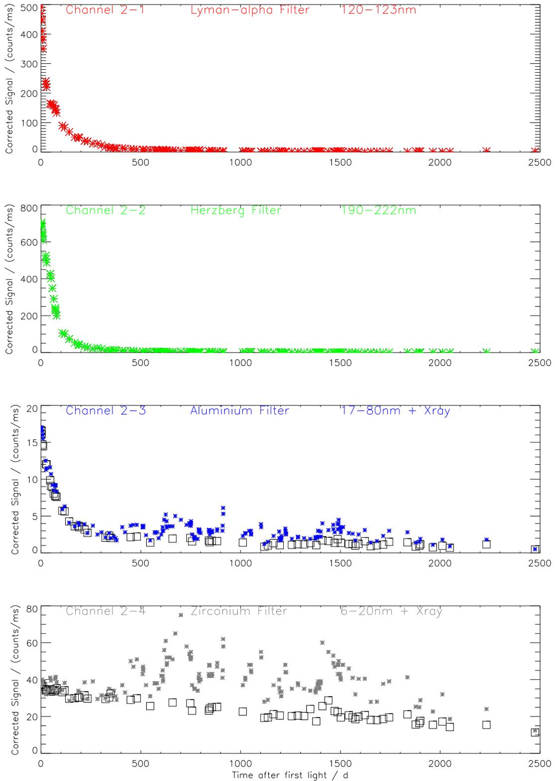
Figure 3: Evolution of unit 2 signal before (stars) and after (squares) removing the solar activity contribution.
