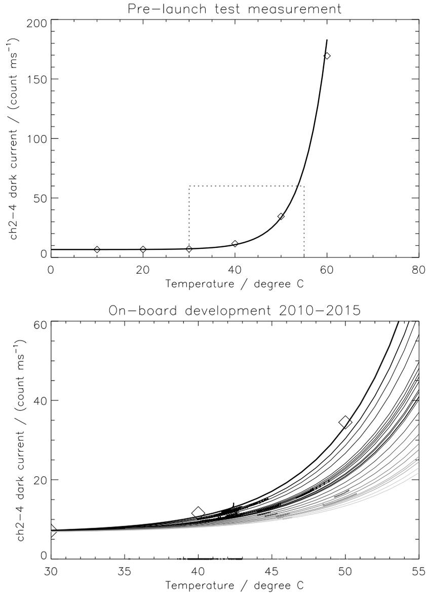
Figure 5: Pre-launch measurement (top panel) and time evolution (bottom panel) of the dark current sensitivity to temperature for the Zirconium channel of Unit 2. The lighter colors correspond to more recent measurements. The temperature range of the bottom panel is highlighted by a dashed rectangle in the top panel.
