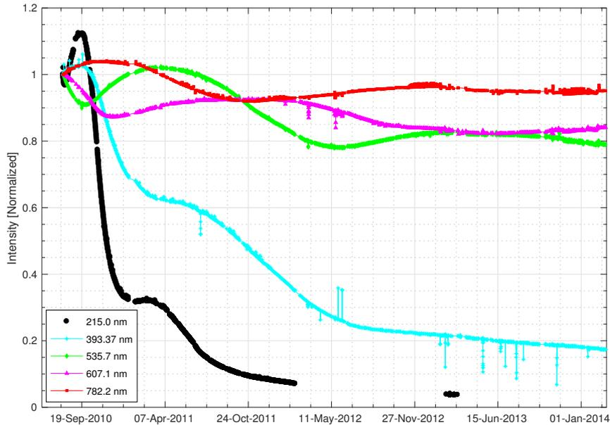
Figure 10: Evolution of the PICARD/SODISM degradation over the full mission.
