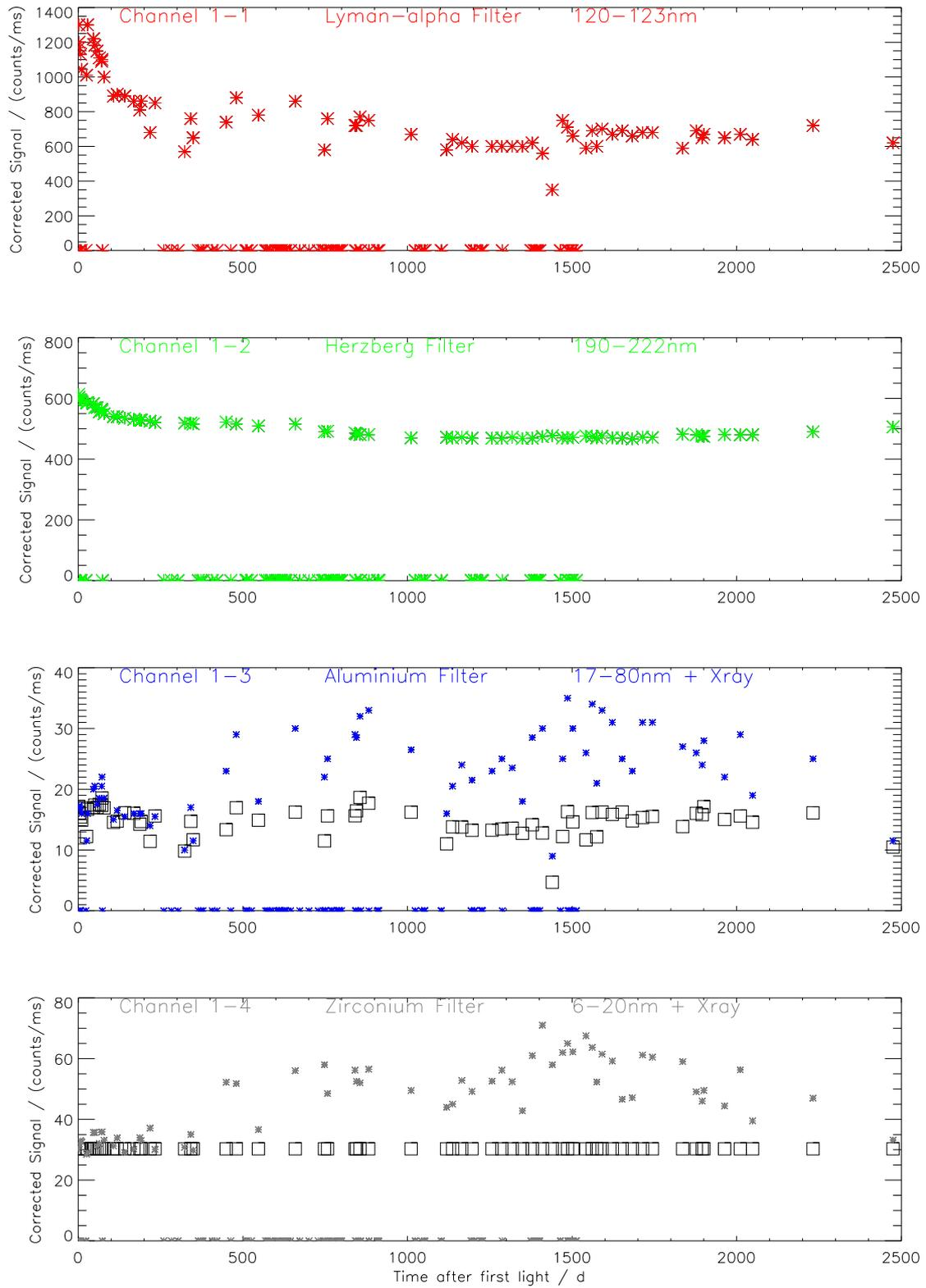
Figure 2: Evolution of unit 1 signal before (stars) and after (squares) removing the solar activity contribution.
