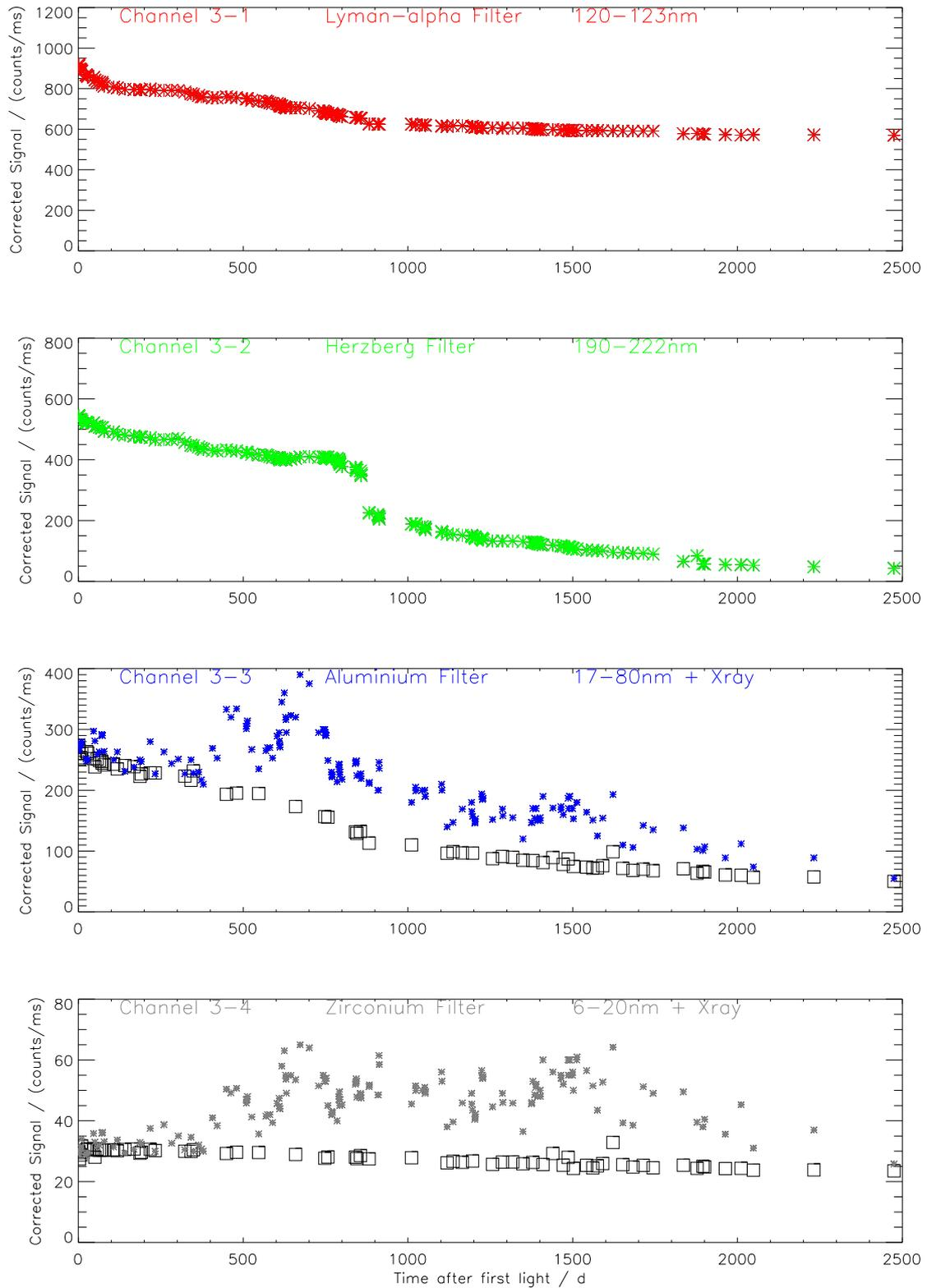
Figure 4: Evolution of unit 3 signal before (stars) and after (squares) removing the solar activity contribution.
