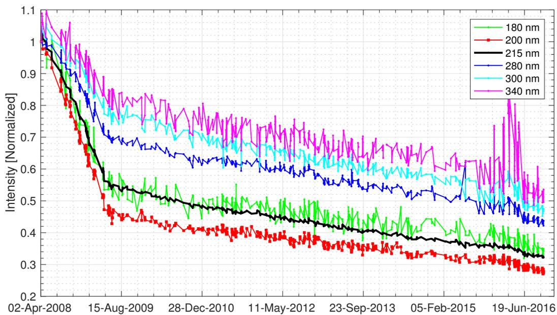
Figure 7: Evolution of the SOLAR/SOLSPEC degradation with time for different UV wavelengths. The temperature of the SOLAR/SOLSPEC instrument can influence the evolution of the signal over time.
