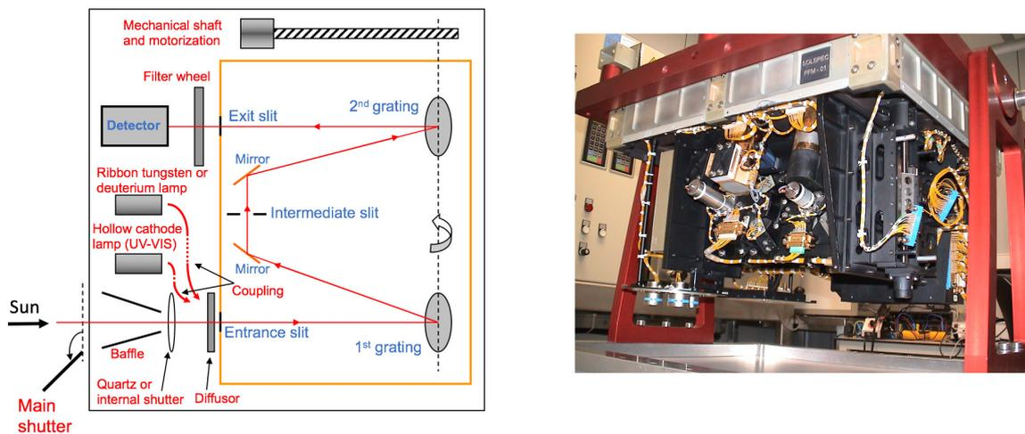
Figure 6: (left) SOLAR/SOLSPEC optical path of one spectral channel (double monochromator). (right) The SOLAR/SOLSPEC instrument with its three units during integration.
