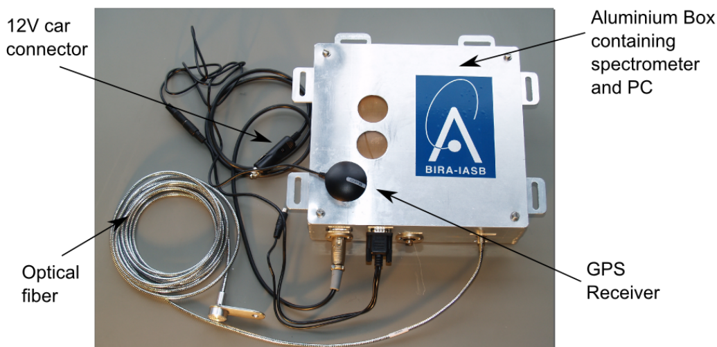
Figure 6.2: The ULM-DOAS instrument. Inside the box are a compact UV-Vis spectrometer and a PC-104. Light is collected directly by the optical fiber and a GPS is used to geolocalize the measurements. The whole system is powered with 12 V.
