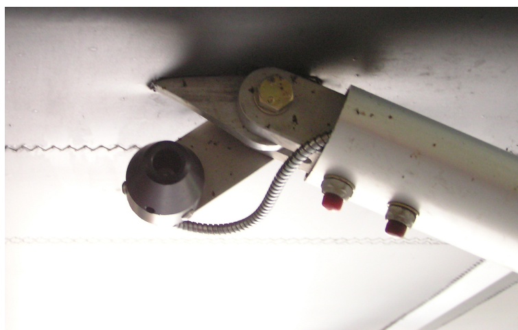
Figure 6.3: Input optics of the ULM-DOAS instrument installed under the wing of the ultralight aircraft. The fiber collects directly the scattered light without any focusing element. The black plastic baffle limits the spatial stray light.
