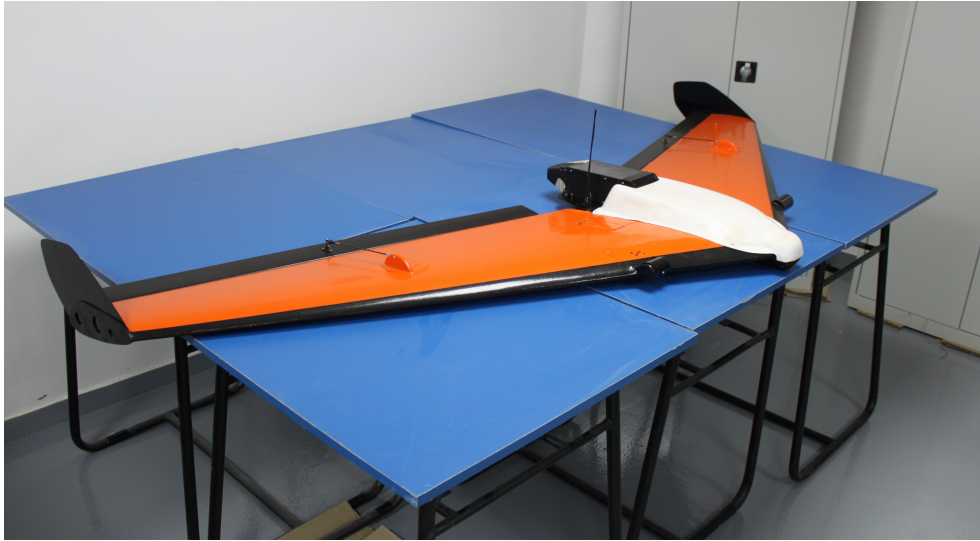
Figure 8.7: The Unmanned Aerial Vehicle built by Reev River Aerospace and dedicated to the SWING payload. It is electrically-propelled and can reach 3 km altitude with its 2.5 m wingspan. The typical speed is 60 km/h.
