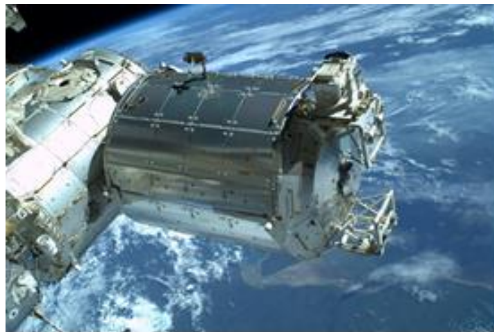
Fig. 1 The European Columbus module on the ISS with the SOLAR payload in view of the external platforms of Columbus. [credits ESA/NASA]
