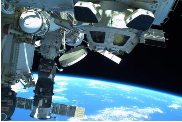
Figure 3: The Cupola (foreground) and Pirs module with the port window (background). [Credit: ESA/NASA]
