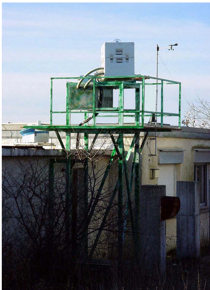
Figure 2: BIRA-IASB UV-visible spectrometer operated at OHP. Alternate observations of the zenith-sky and of the “off-axis” scattered light ( 10^\circ above horizon) are obtained by means of a rotating mirror installed in a quartz dome on top of the box.
