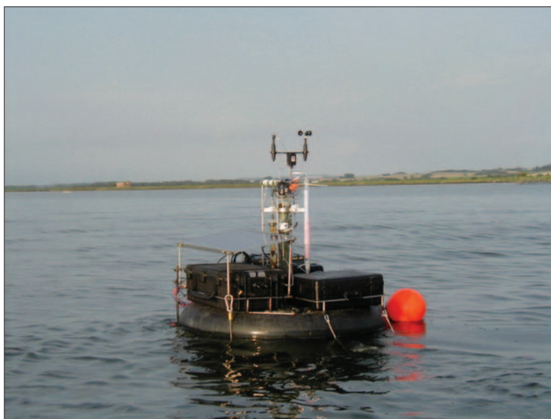
Figure 3.3 - Floating Equilibrator System deployed in the Randers Fjord (Denmark). This device continuously monitors the CO 2 concentration of surface water, together with temperature, salinity, and meteorological parameters such as wind speed, air temperature, and solar irradiance. It is powered by batteries and a solar panel and includes an infrared spectrometer for CO 2 determinations. (ULg-OCEANCHEM).
