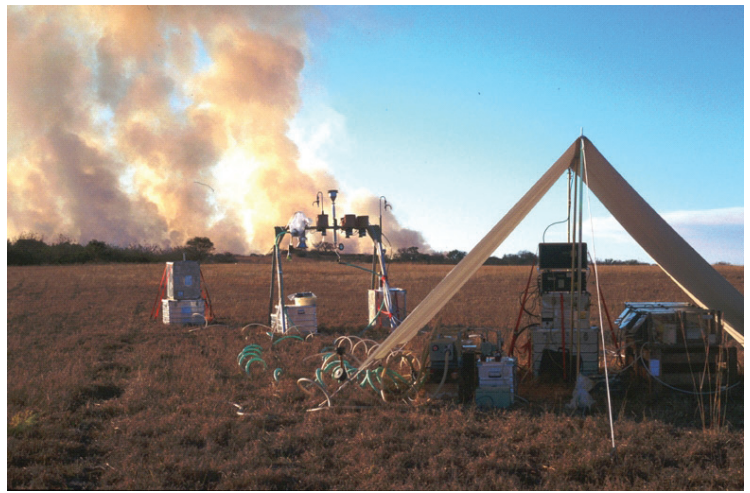
Figure 1.19 - Aerosol sampling set-up used during SAFARI 2000 in the Kruger National Park, South Africa. (W. Maenhaut, UGent-INW).
