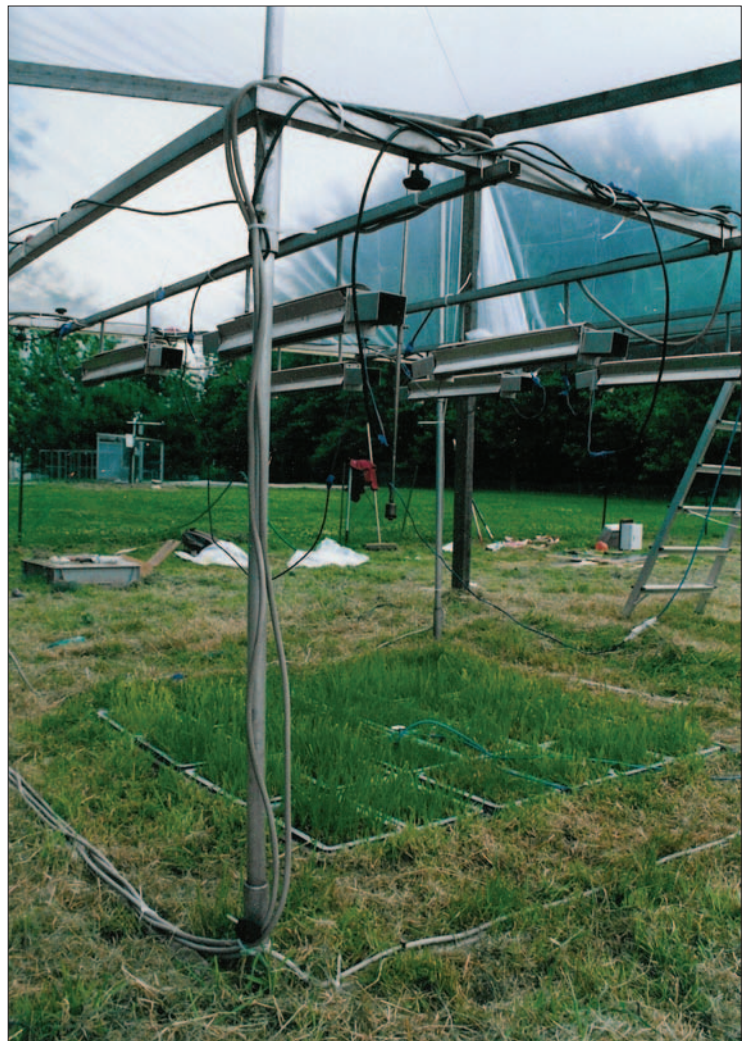
Figure 4.1- Simulation of natural heat waves with suspended infrared heaters (Free Air Temperature Increase technique) at UA. Below the heaters are containers with artificially composed grassland communities with different numbers of plant species, to verify whether loss of plant diversity affects sensitivity to extreme events. (I. Nijs, UA-PLECO).
