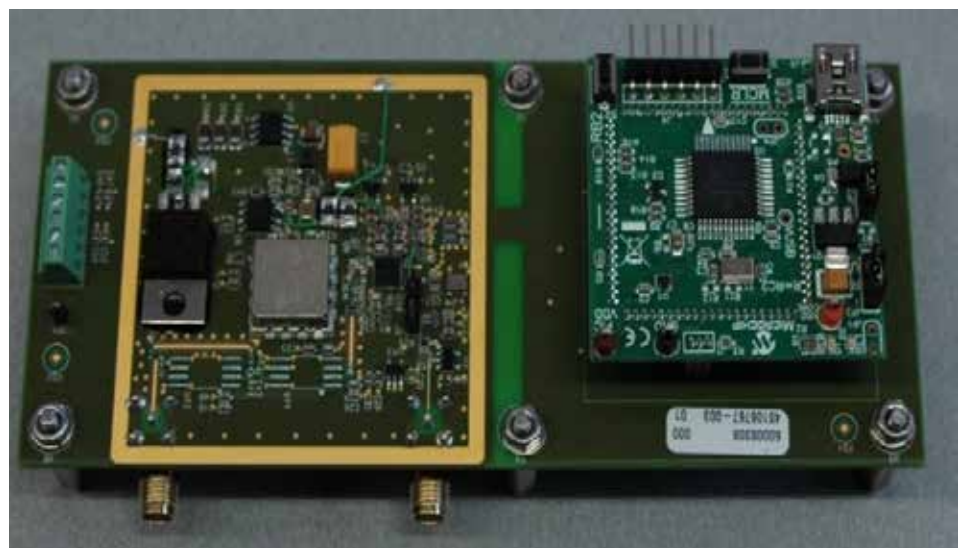
Figure 9 — Picture of the assembled PCB containing the PLL chain, power handling and PIC.
