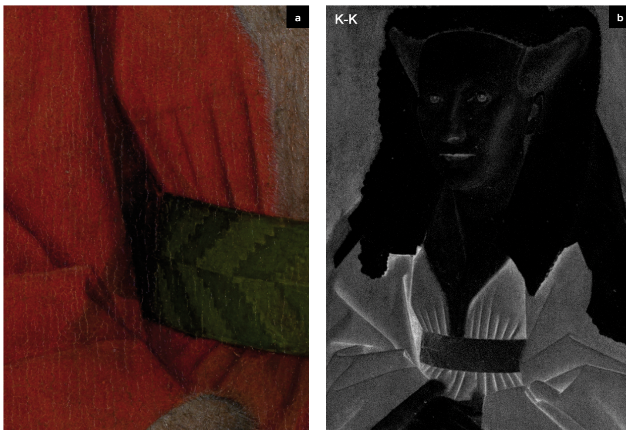
Figure 7. (a) Detail of the area between the sitter's arm and belt in normal light. (b) Elemental map of potassium.
