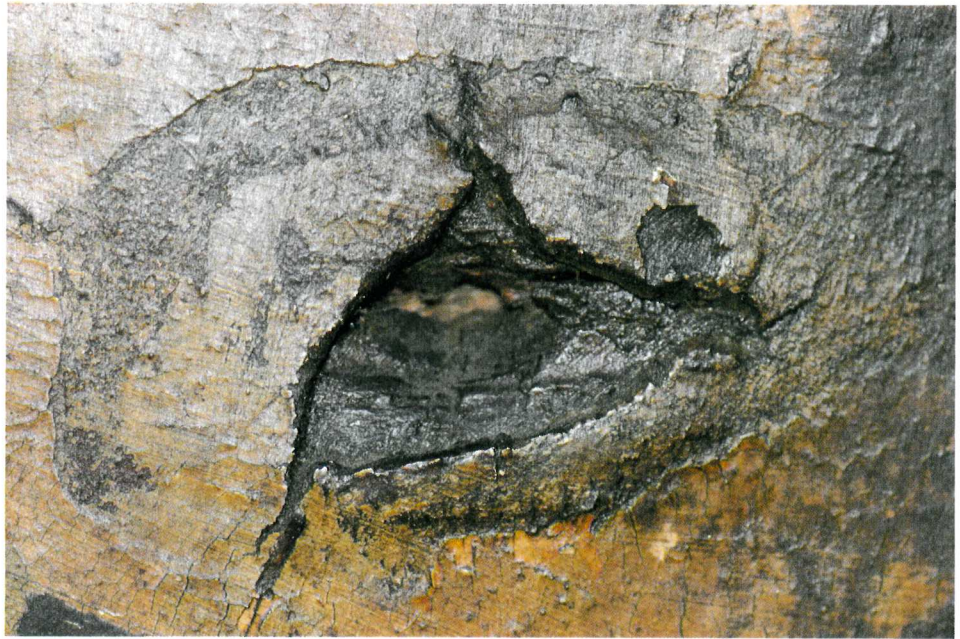
Figure 11 Unrepaired impact damage from a pointed object. © C. Currie
