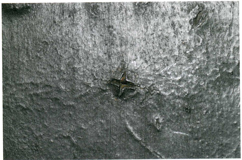
Figure 10 Cross-shaped impact damage in leather in the 3rd plank from top just above drawbridge. © C. Currie
