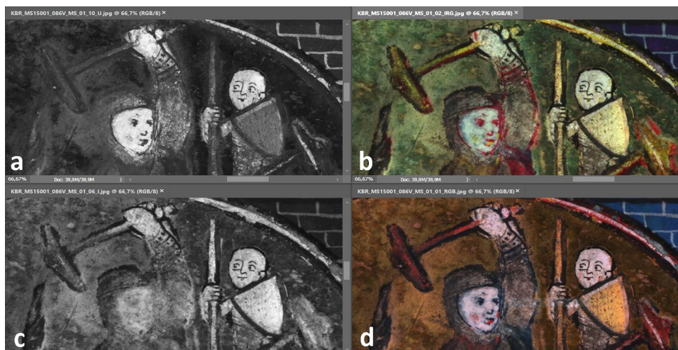
Fig. 4. A MS MicroD result on a detail on folio 86v: (a) UV reflectance, (b) tri-chromatic infrared-red-green (IRG) false colour rendering, (c) NIR reflectance, (d) standard tri-chromatic red-green-blue (RGB) visual representation.
