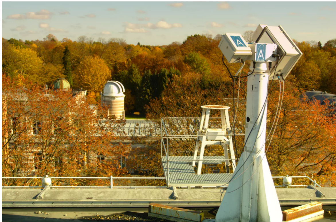
Figure 7.1: Picture of the MAX-DOAS instrument at Uccle, Belgium (Source: A. Merlaud).
